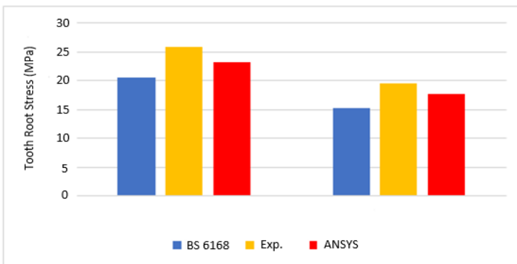
Figure 6. Comparison of analytical, BS6168 standard and ANSYS tooth root stress results
