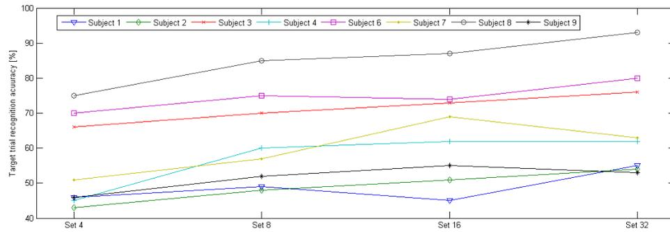
Figure 2: Disabled subjects 1-4 and able-bodied subjects 6-9. Increasing number of electrodes result in higher target trial recognition accuracy.
