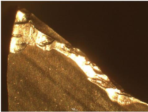
Fig 6: Tool flank wear for treatment 24 m/min and 0.15 mm/rev
