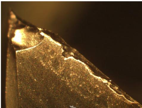
Fig 10: Tool flank wear for treatment 30 m/min and 0.15 mm/rev
