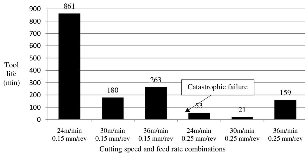
Fig 5: Tool life for different cutting speed and feed rate combinations
