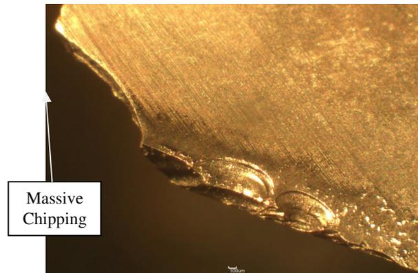
Fig 12: Tool rake for treatment 24 m/min and 0.25 mm/rev
