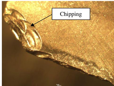
Fig 11: Tool rake for treatment 30 m/min and 0.15 mm/rev
