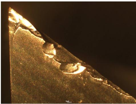
Fig 8: Tool flank wear for treatment 30 m/min and 0.25 mm/rev
