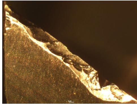
Fig 7: Tool flank wear for treatment 36 m/min and 0.15 mm/rev
