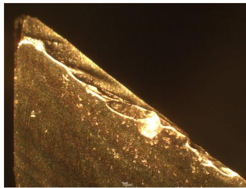
Fig 9: Tool flank wear for treatment 36 m/min and 0.25 mm/rev
