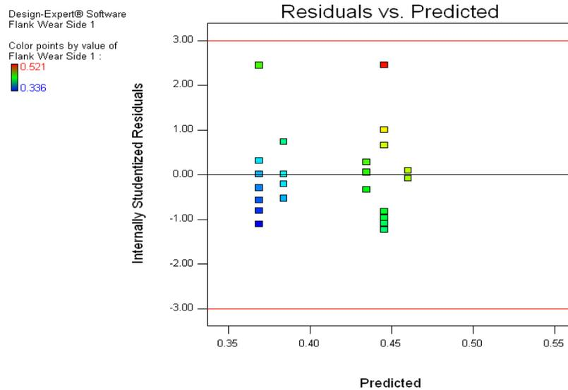
Fig 3: Constant variance in data for flank wear side 1.
