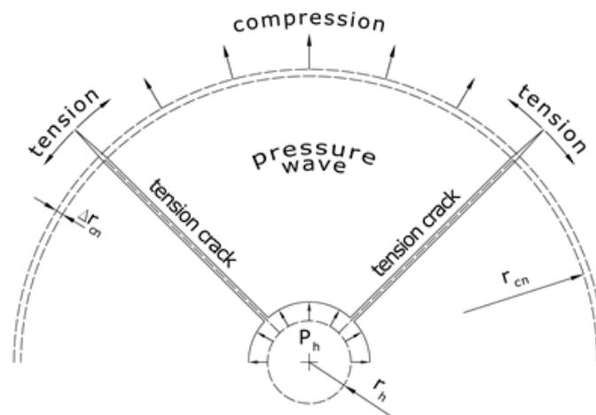
Figure 2 Schematic illustration of rock blasting model
