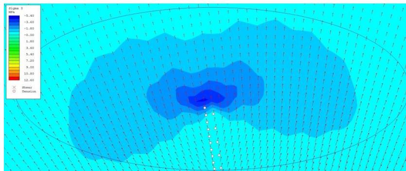
Figure 6 Contours of minor principal stress with deformation vectors
