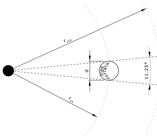
Figure 9 The distance between the empty and charged cut hole
