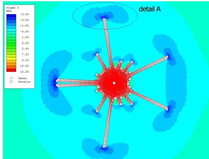
Figure 4 Contours of minor principal stress with yielded elements
