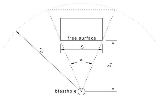
Figure 10 The distance from blast hole to limited free surface
