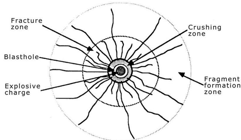
Figure 1 Schematic illustration of processes occurring in the rock around a blast hole, showing formation of crushing zones, fracture zones and fragment formation zone
