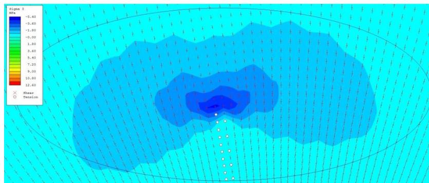
Figure 5 Contours of minor principal stress with principal stress trajectories
