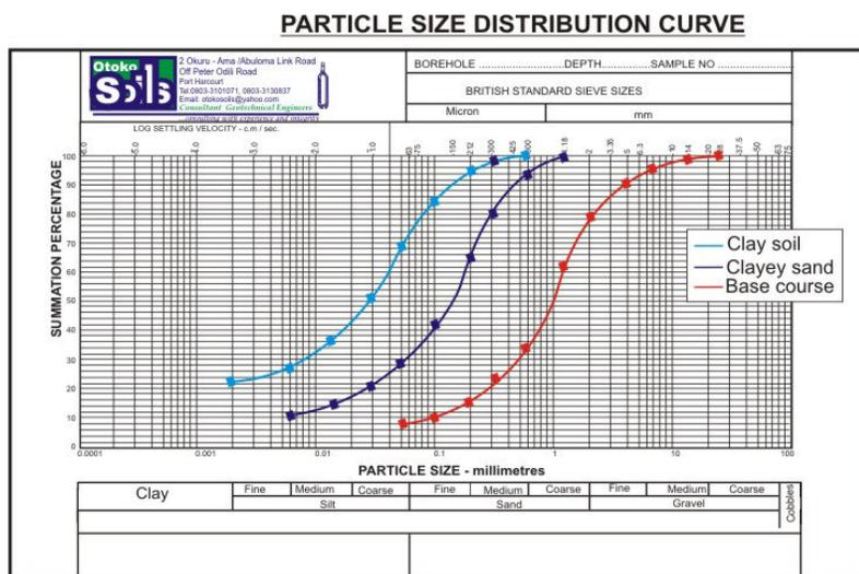
Fig 2 Particle size distribution curves of clay soil, clayey sand and base course.
