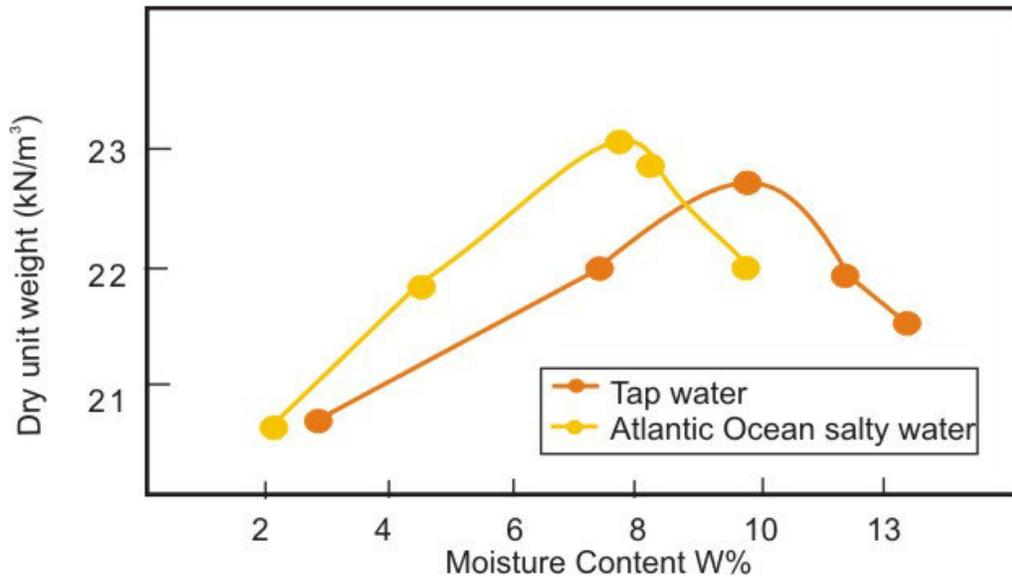
Fig 5. Compaction curves for base course using tap water and Atlantic Ocean water
