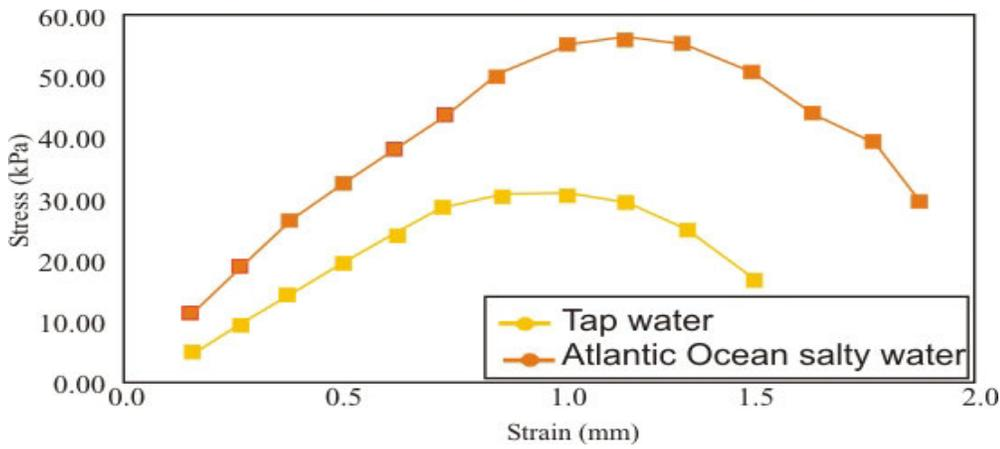
**Figure 6.** Stress Strain relation for clay soil with tap water and Atlantic salty water.
