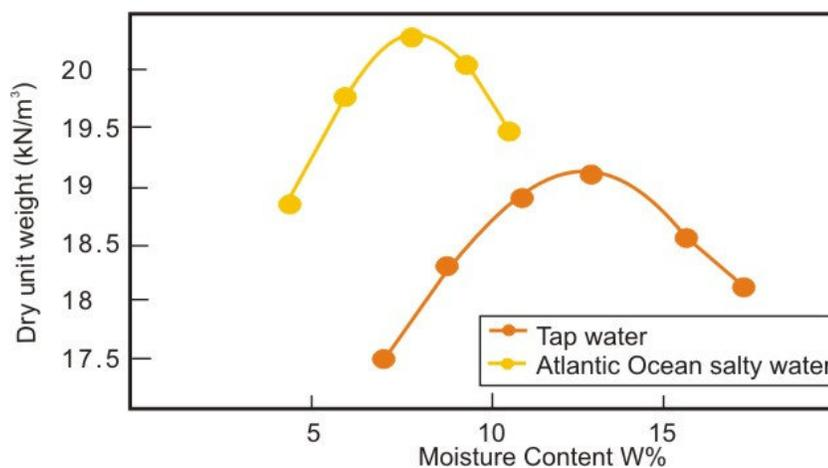
**Fig 4.** Compaction curves for clayey sand using tap water and Atlantic Ocean water
