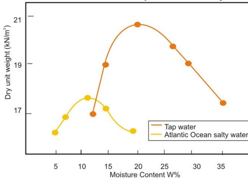
**Fig 3.** Compaction curves for clay soil using tap water and Atlantic Ocean water
