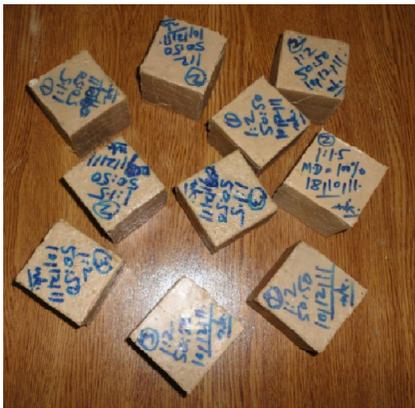
Figure 3 Test specimens after casting being cured at room temperature
