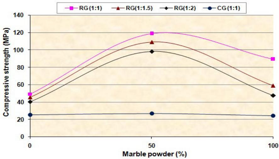
Figure 5 Compressive strength of CG and RG versus proportion of marble powder
