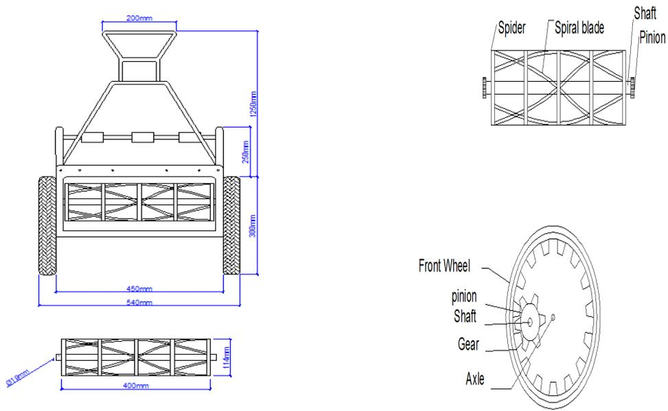
Figure 2. Shows the driving arrangement.
