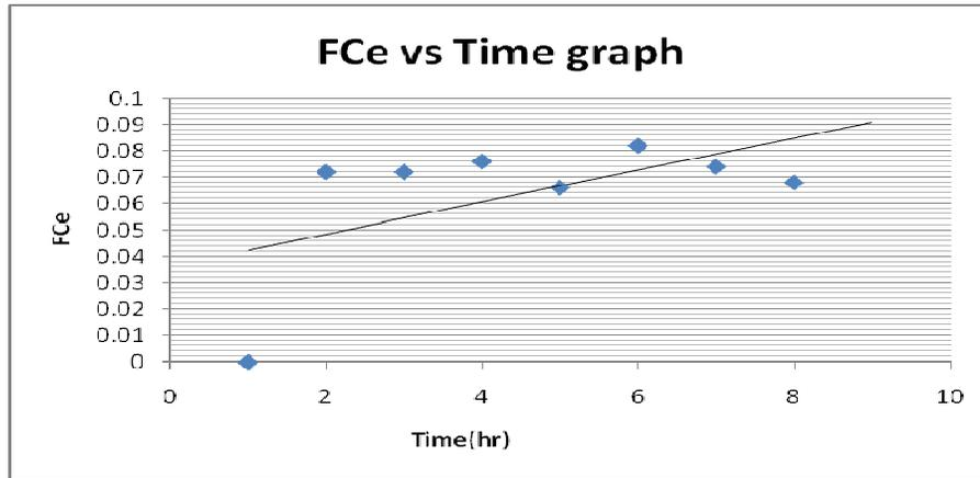
Figure 4: The relationship between the effective capacity and operational time.
