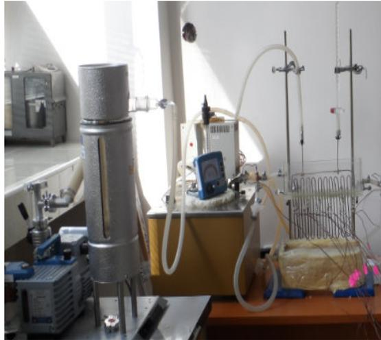
**Fig. 3 Pumping air through a pump and filling pulsating heat pipes**
