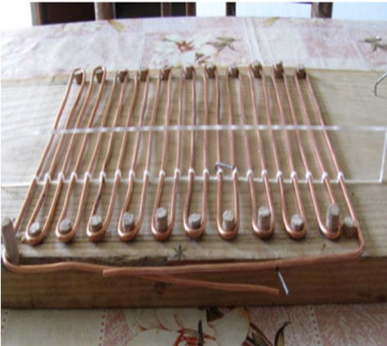
**Fig.2 Closed loop pulsating heat pipe**
