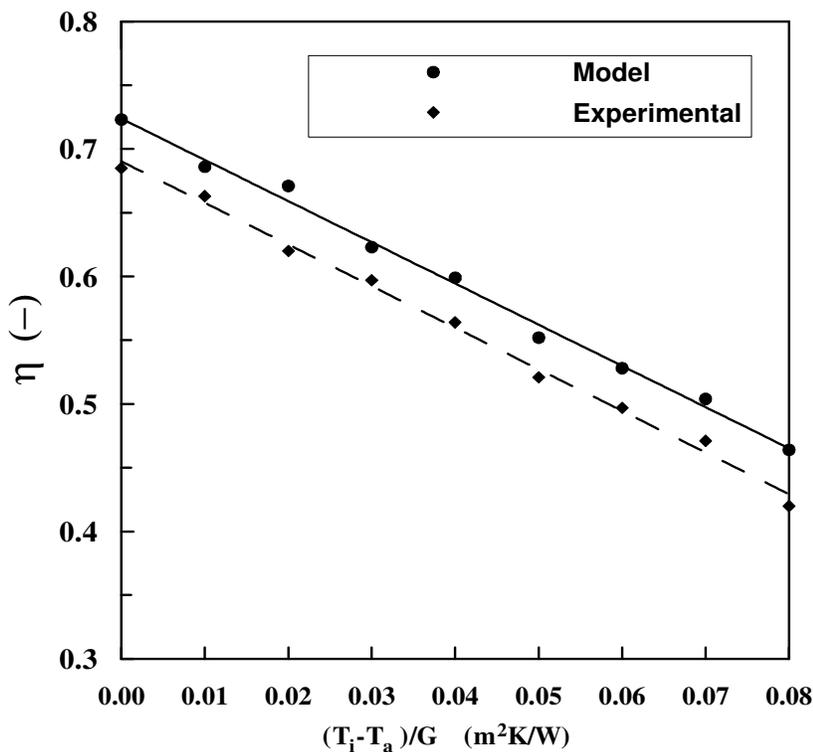
**Figure 3. Comparison between simulated and experimental ETC thermal efficiency**
