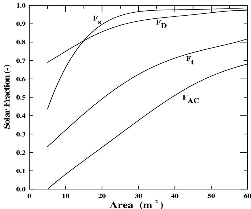
Figure 4. Solar fraction variation with collector area
