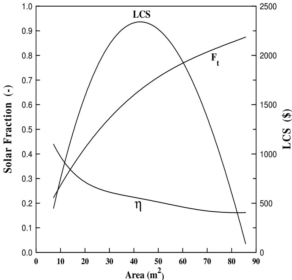
Figure 5. Variation of system parameters with collector area
