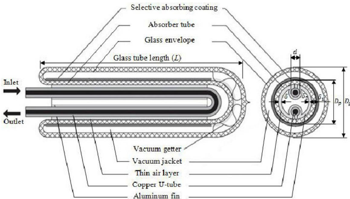
**Figure 1. Schematic diagram of the glass evacuated tube solar collector with U-tube**
