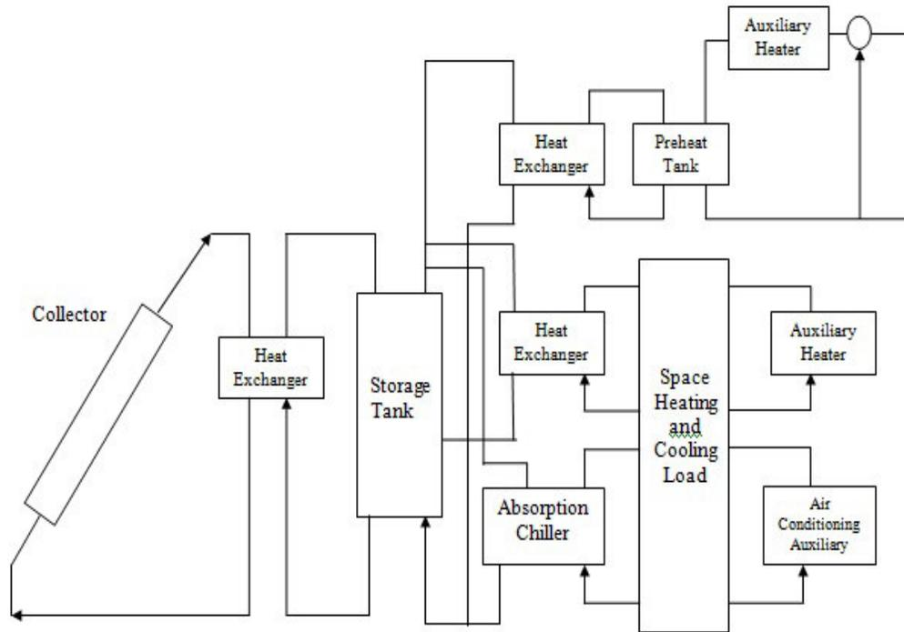
**Figure 2. Schematic diagram of the solar heating and cooling system**
