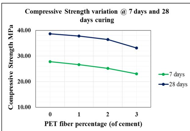
Figure 5: Effect of PET fibers on the Compressive Strength of concrete at 7 and 28 days.
