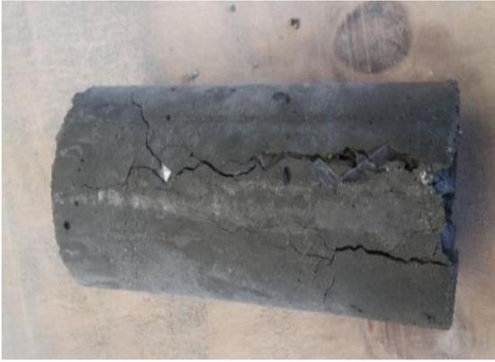
**Figure 7: Concrete cylinder with PET fibers after splitting tensile strength test**
