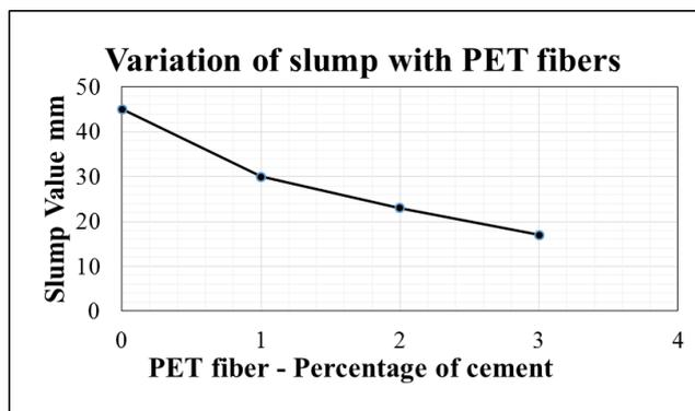
**Figure 3: Variation of slump with PET fibers**
