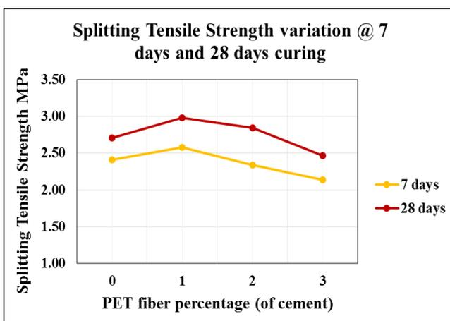
Figure 6: Effect of PET fibers on the Splitting Tensile Strength of concrete at 7 and 28 days.
