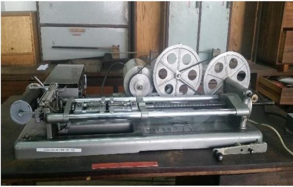
**Figure 2: Tensometer machine for testing Tensile Strength of the PETfibers**
