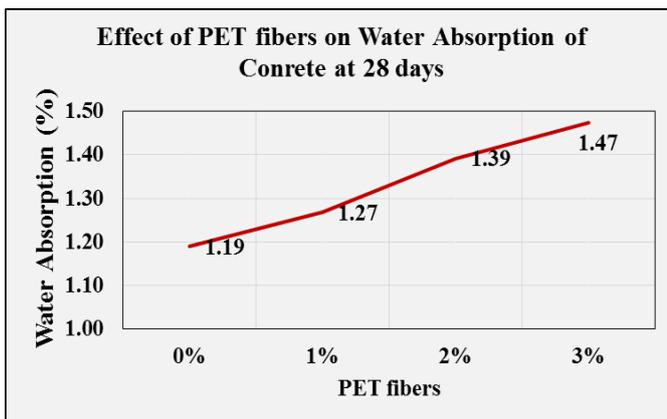
Figure 4: Effect of PET fibers on the water absorption of concrete at 28 days.
