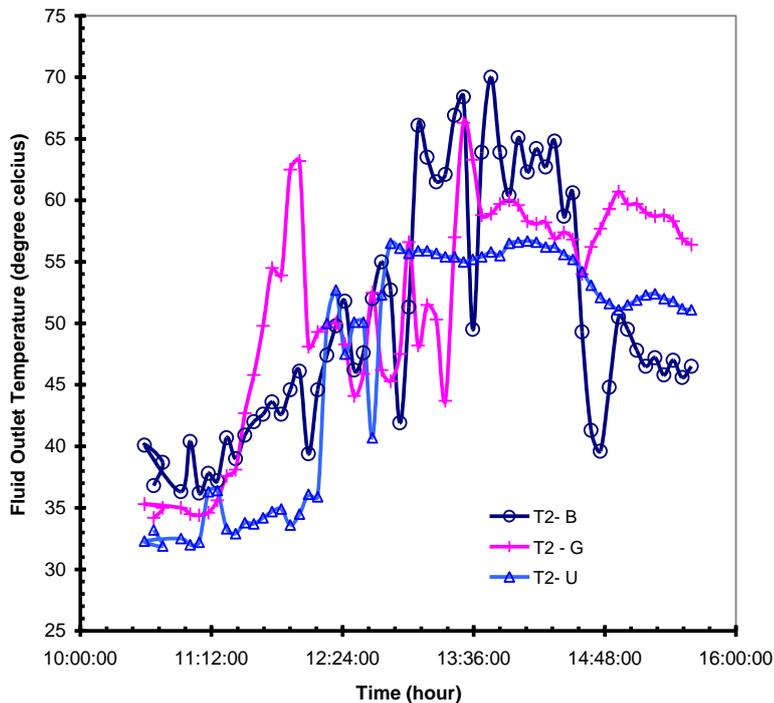
**Fig 5 Fluid Outlet Temperature of the receivers against time**
