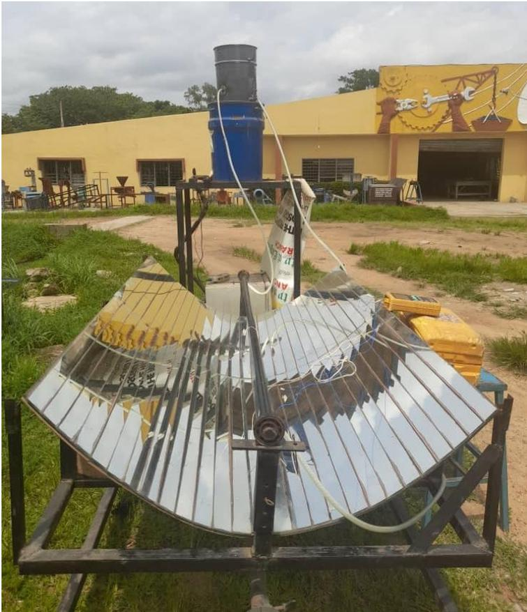
**Figure 1: The parabolic trough system with storage tank**
