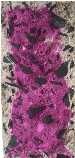
**Fig. 5** Example of cylindrical specimens after ruptured and sprayed with phenolphthalein solution
