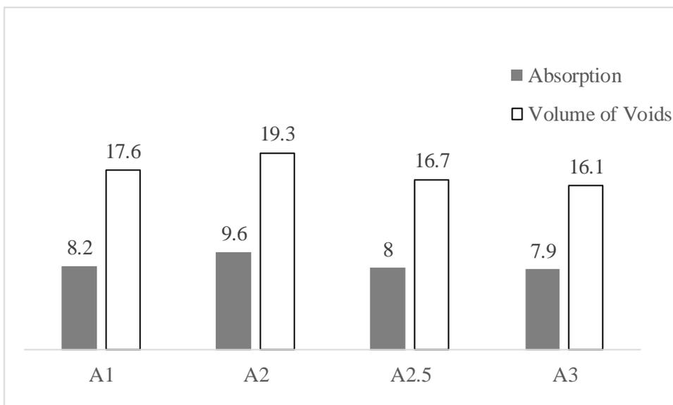
**Fig. 8** Absorption after immersion and Volume of Voids (%) obtained from samples
