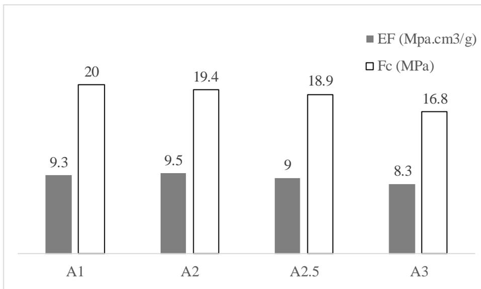
**Fig 6** Compressive Strength  $F_c$  (MPa) and Efficiency Factor EF (MPa.cm<sup>3</sup>/g) obtained from samples
