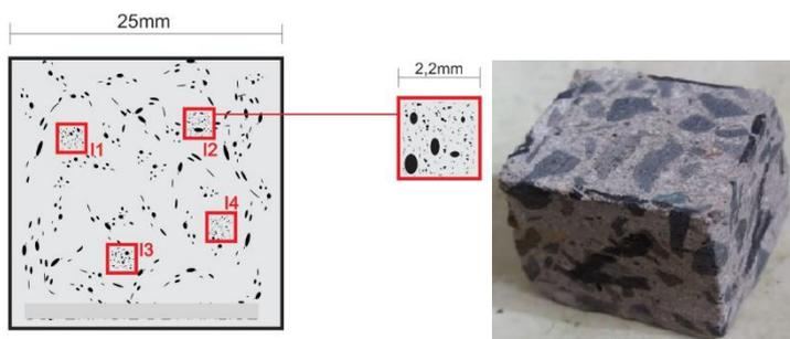
**Fig. 3** Example of cubic specimens for the optical microscope
