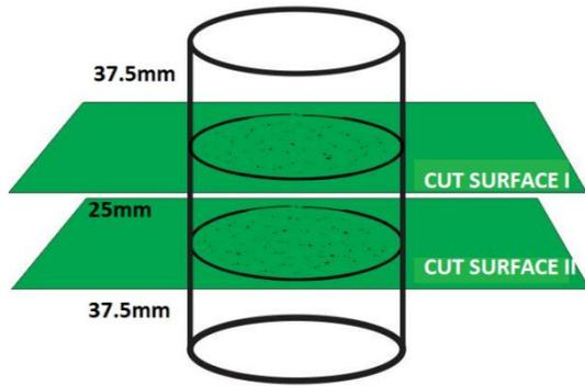
**Fig 1** Cut surfaces by circular saw
