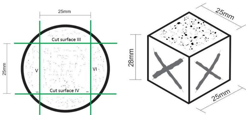
**Fig 2** Cut surfaces by circular saw
