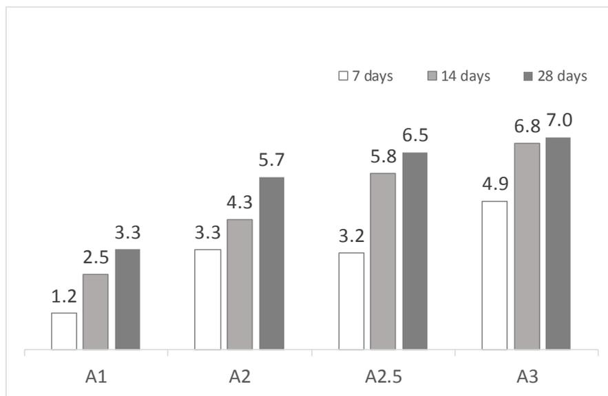
**Fig. 9** Carbonation Front Depth (mm) of the samples at 7, 14 and 28 days under Accelerated carbonation process
