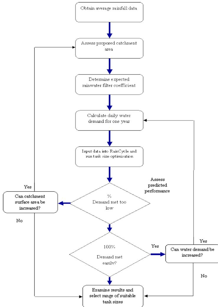
Figure 3 Determining range of suitable tank sizes
