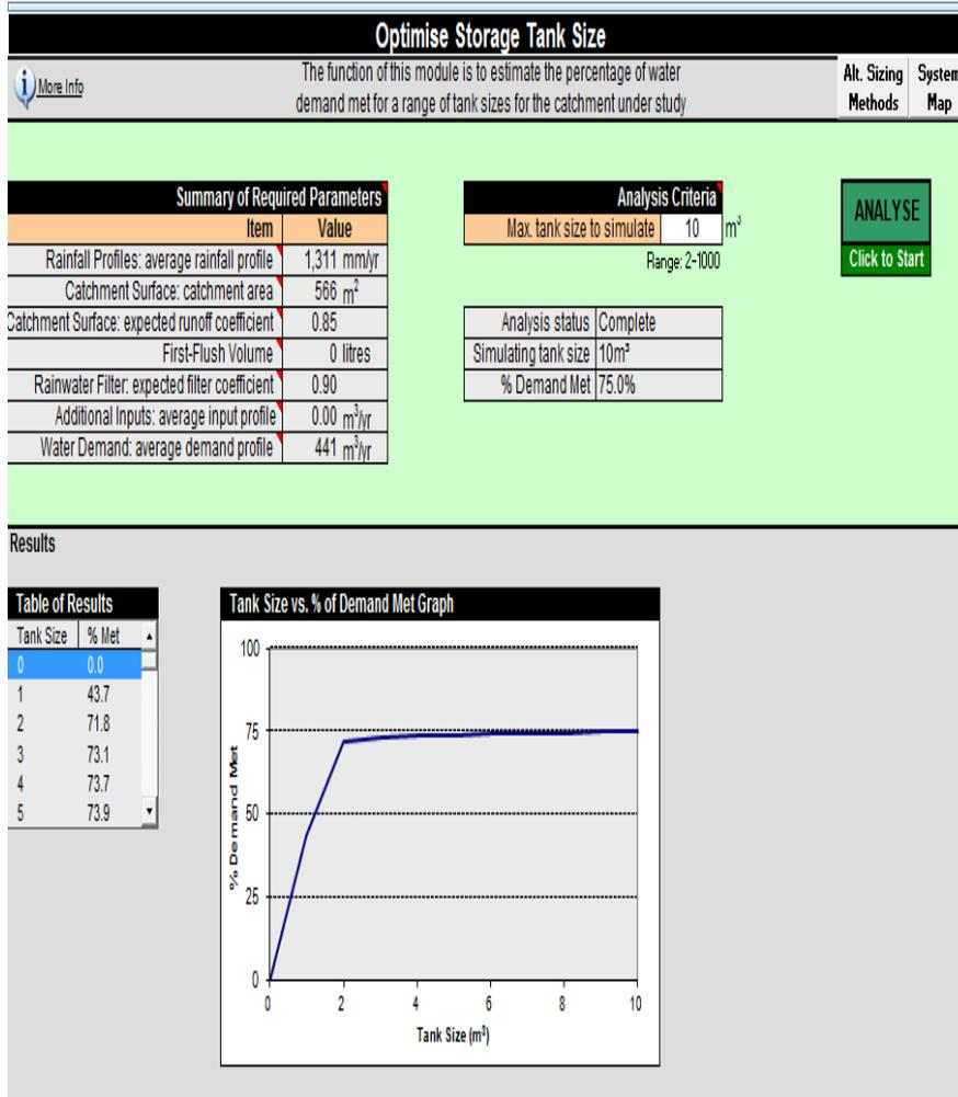
Figure 4 Results from optimising tank size.
