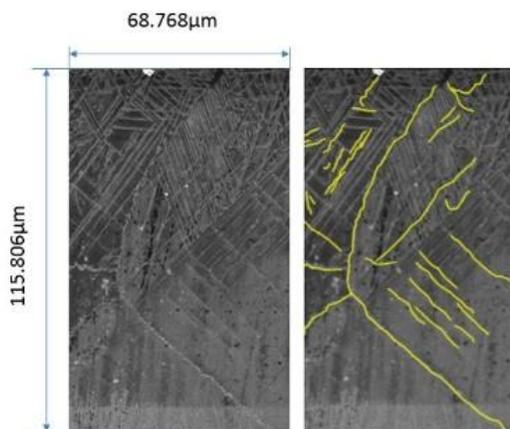
**Fig 6.** Location of dislocations in a section of the sample analyzed.
