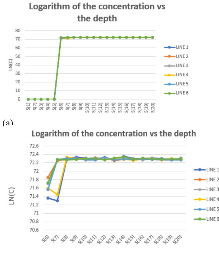
**Fig. 9** a) Logarithm of concentration as a function of depth for the zone of dislocations, b) points for the regression.
