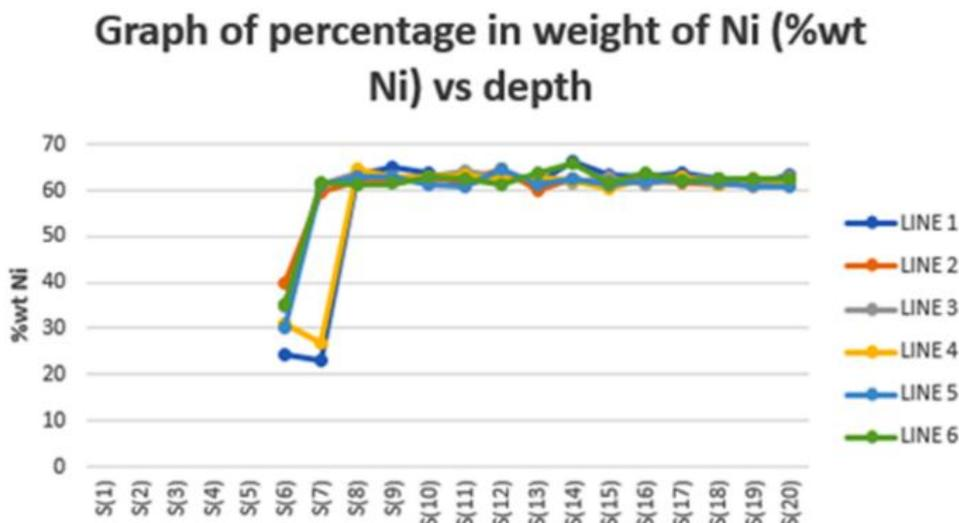
**Fig.8** Graph of percentage by weight of nickel in the zone of the dislocations. The total depth analyzed was 15 μm.
