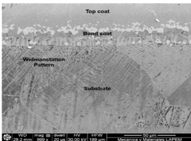
**Fig. 3** The UDIMET 500 substrate micrograph 999x.
