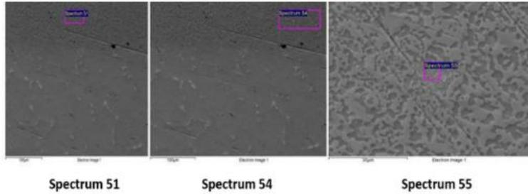
**Fig.4** Micrograph obtained after of energy dispersion analysis by spectroscopy in the bond coat section, the inspection area is inside the rectangle.
