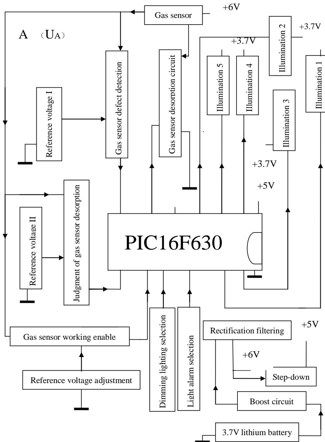
Fig.3. Circuit schematic diagram
