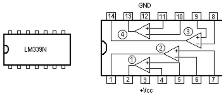
**Fig.1. LM339 interface diagram**
