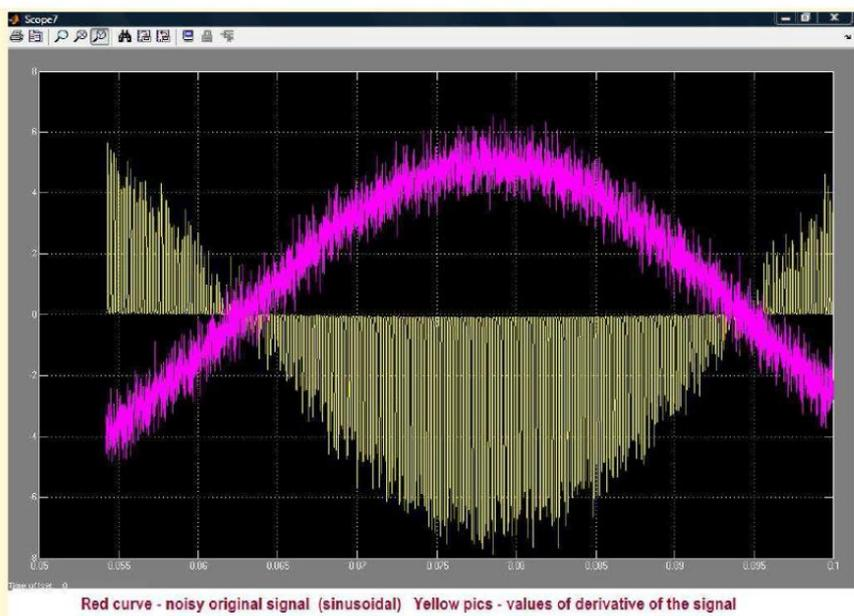
**Figure 5.** Signal 100 rad/sec and its derivative.
