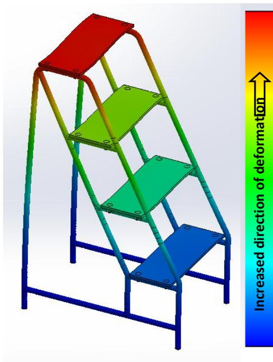
Figure 6: Buckled shape due the application of load on the top step
