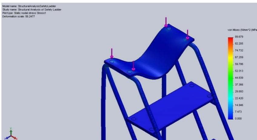
Figure 3: Static analysis: distribution of stress on the top step
