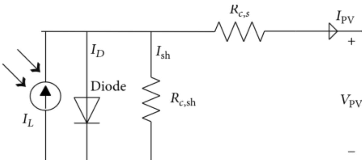
**Figure 1: The one-diode model equivalent**
