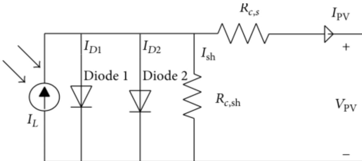
**Figure 2: The two-diode model equivalent**
