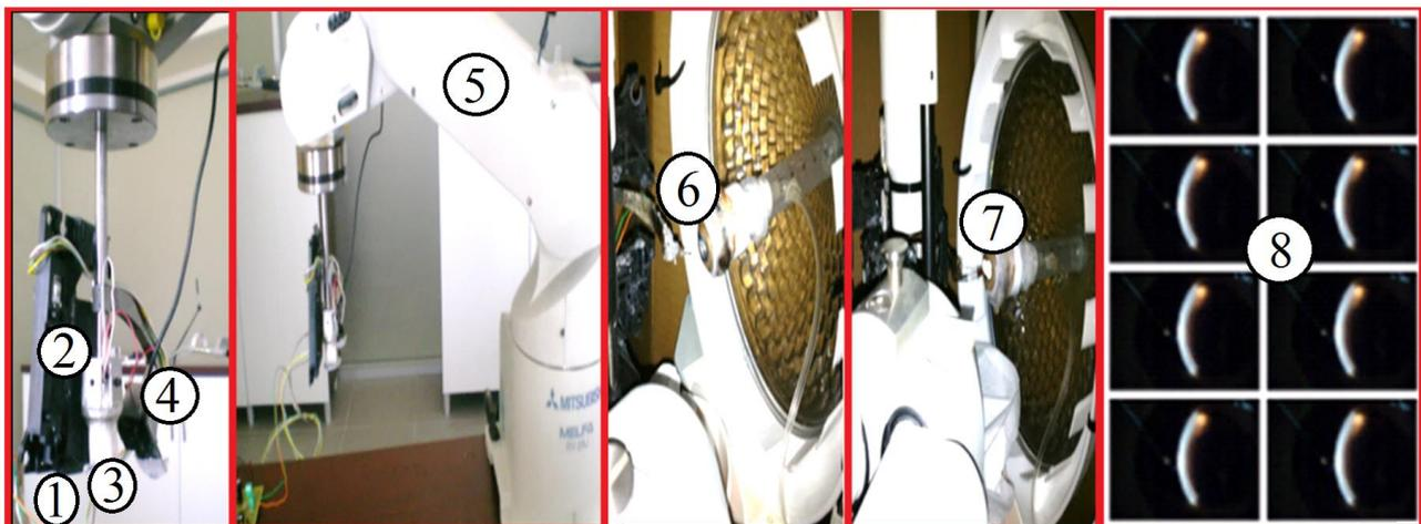
**Figure 11: Mechatronic structure of corneal elasticity measurement system.**
