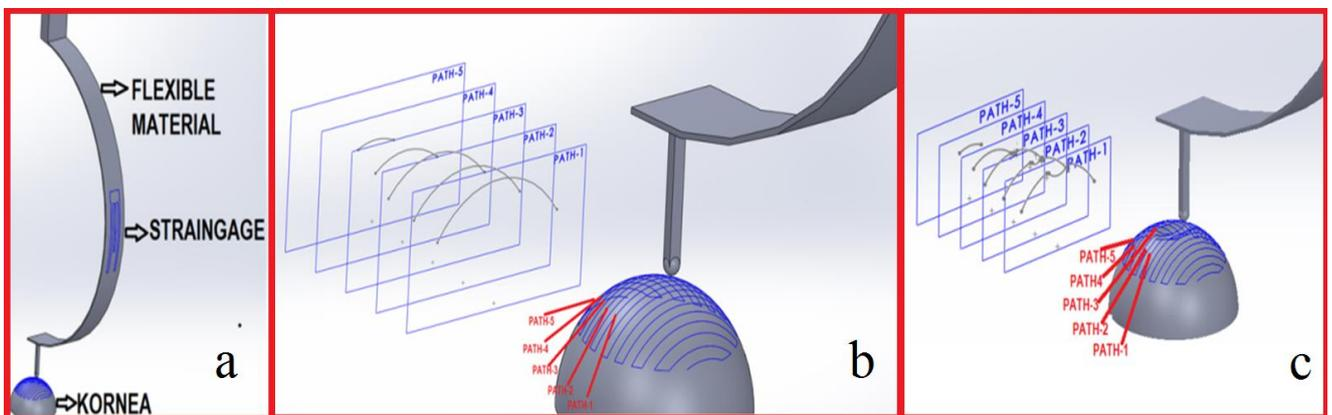
**Figure 12: ESKIS measurement system** a: measurement apparatus, b: Sample measurement for healthy eye, c: measurement example of structural change in the eye.
