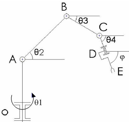
**Figure 10: Kinematic model of Mitsubishi RV-2AJ**
