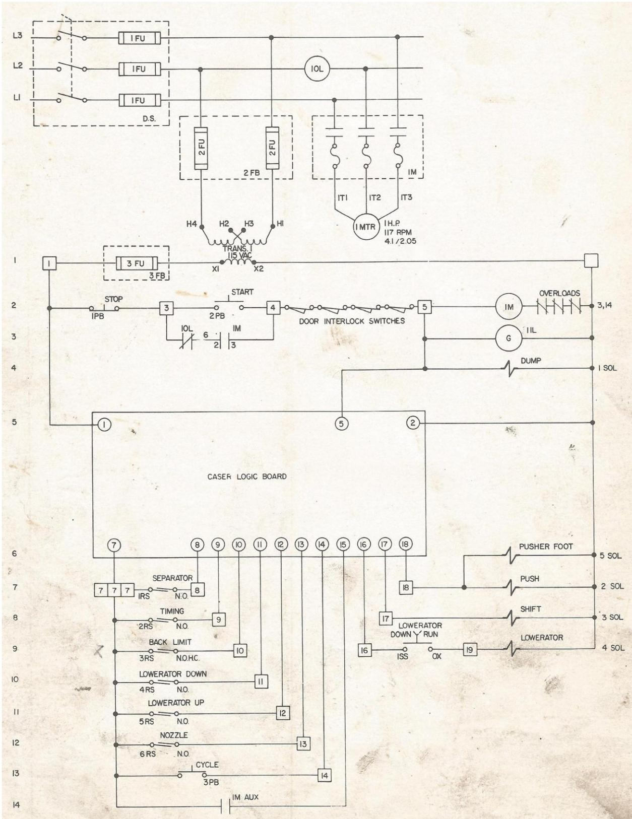
Fig.3: Electrical schematic
