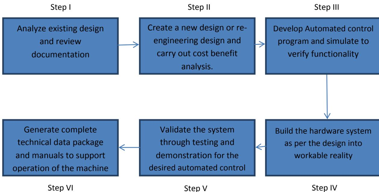
**Fig.1: Step by Step Approach for retrofitting of machine**
