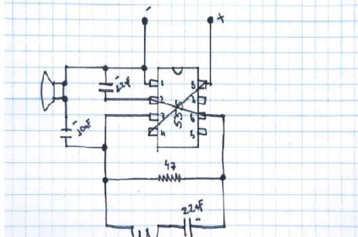
Figure1 – Electrical circuit of the homemade metal detector.
