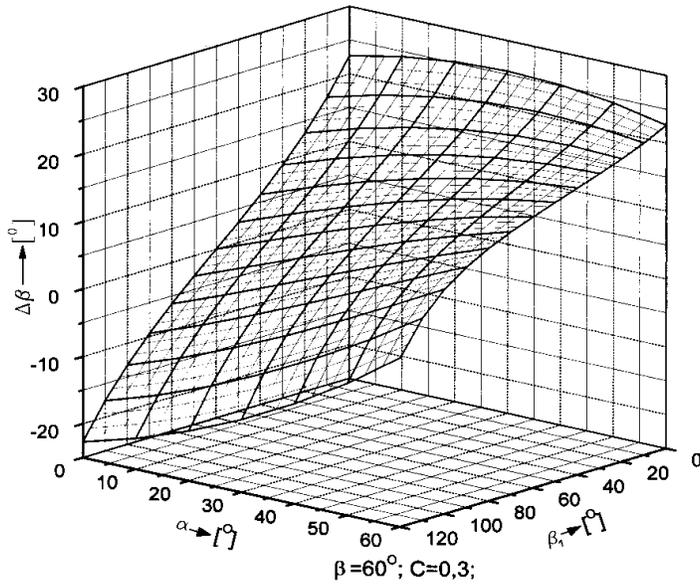
FIGURE 8. Dependence of the angle  $\Delta\beta$  on the flight position angle and material characteristics
