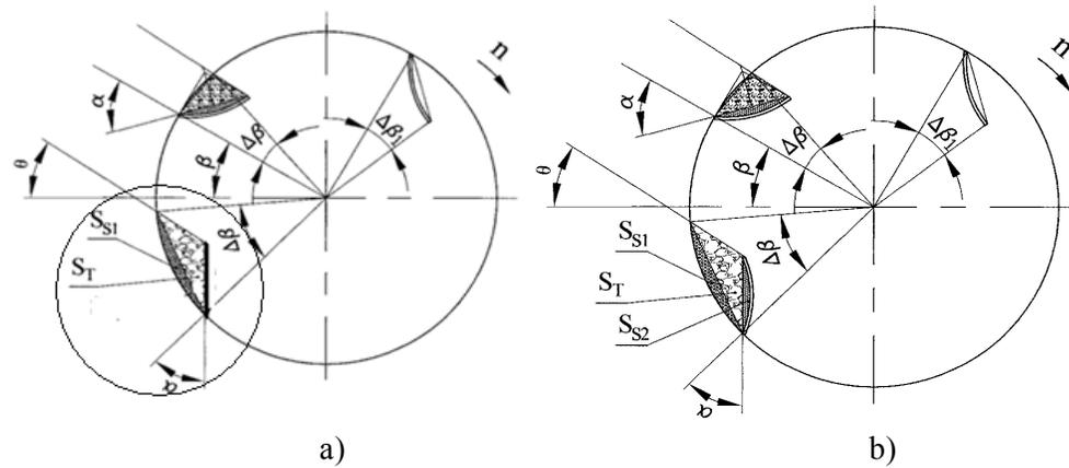
**FIGURE 2.** Scheme for determining the area of the material on the flight (a – of a flat flight; b – of a curved flight)
