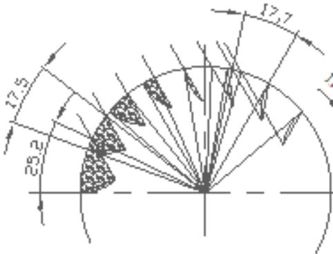
FIGURE 4. Angle of natural repose
