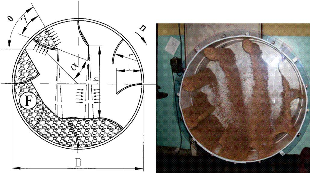
**FIGURE 1.** Cross-section of the drying chamber showing distribution and feeding of the material
