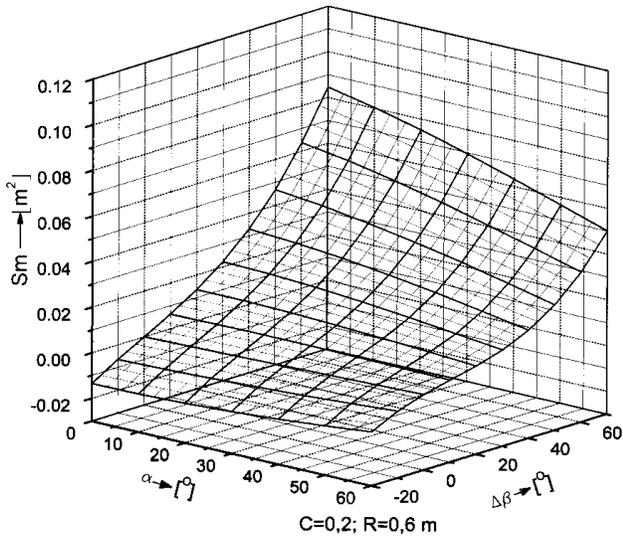
FIGURE 3. Dependence of the material surface on the flight mounting angle
