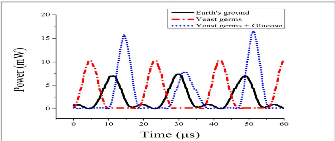
Fig. 4 With an EM radiation from a 4-tube fluorescent lamp as the input signal, the one with Yeast germs (12 beds in series) negative potential ground rectifying shows 60 % more power, and a raise of about 125% was rendered by further feeding the germs with 0.05M glucose solution
