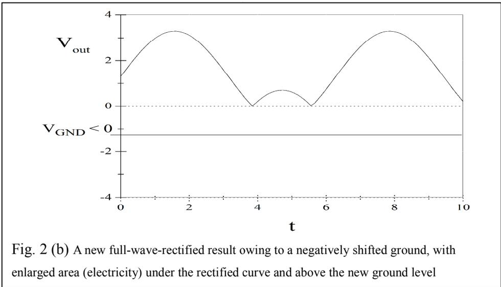
Fig. 2 (b) A new full-wave-rectified result owing to a negatively shifted ground, with enlarged area (electricity) under the rectified curve and above the new ground level
