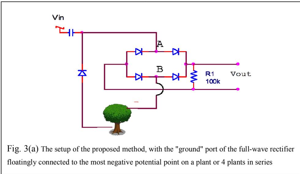
Fig. 3(a) The setup of the proposed method, with the "ground" port of the full-wave rectifier floatingly connected to the most negative potential point on a plant or 4 plants in series
