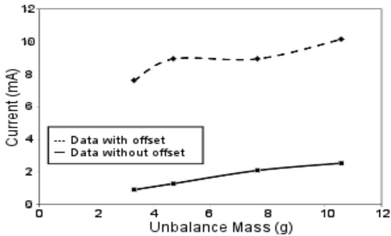
Figure 2. Behavior of harmonics with mechanical unbalance in grams.
