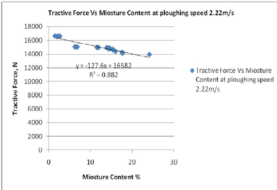
Figure 2 : Effect of moisture content on tractive force at 2.22 m/s tillage speed for ploughing.
