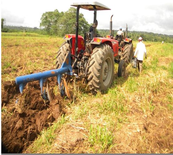
Plate 1. A photograph depicting tractor- dynamometer, implement mounted position during disc ploughing operations.
