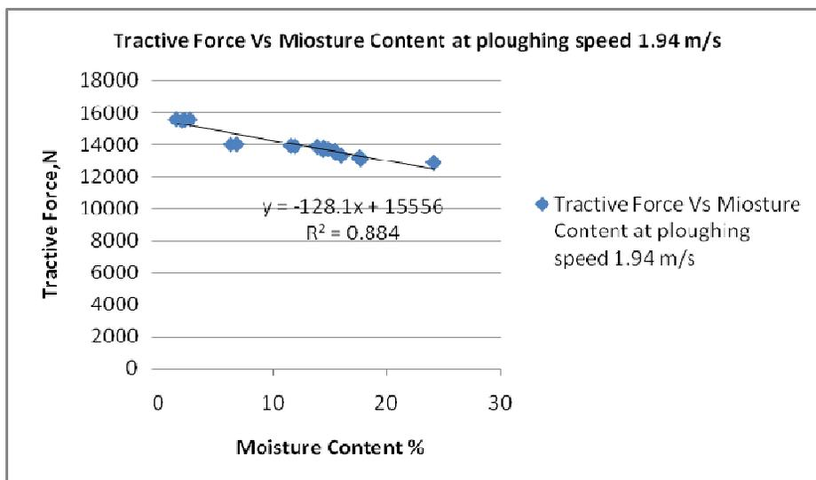
Figure 1 : Effect of moisture content on tractive force at 1.94m/s tillage speed for ploughing.
