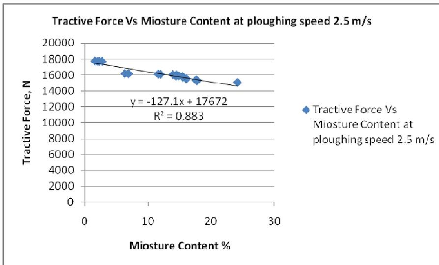
Figure 3: Effect of moisture content on tractive force at 2.5 m/s tillage speed for ploughing.
