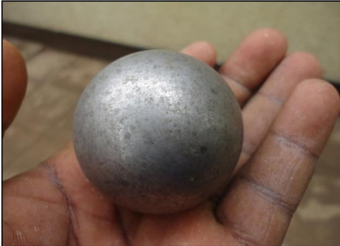
Plate 1: 438g spherical steel bearing
