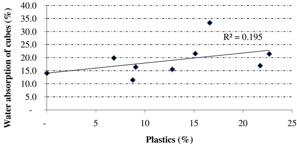
**Figure 7: Effect of plastics (%) on the water absorption of cubes**
