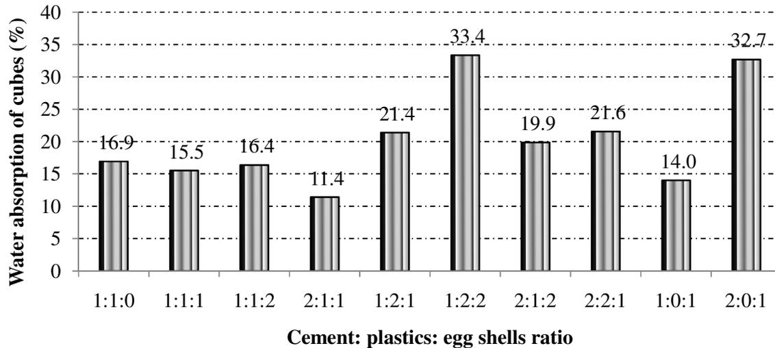
**Figure 5: Effect of mix proportions on water absorption of the cubes**
