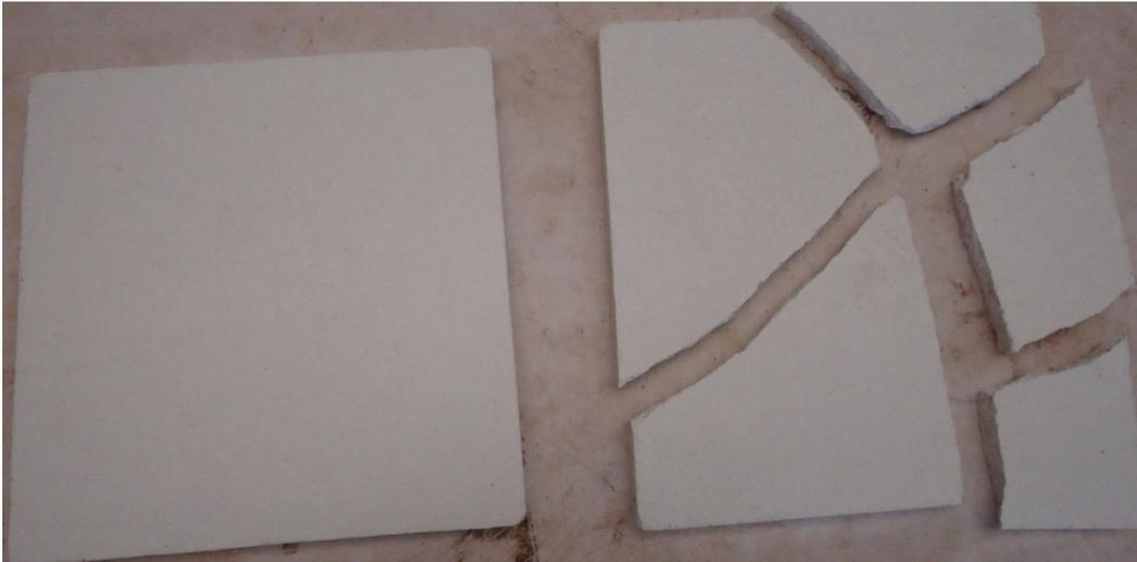
Plate 4: Shattered tile made with cement and egg shells without plastics
