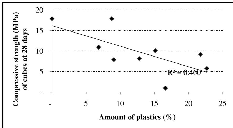
Figure 2: Effect of plastics (%) on the cube compressive strength
