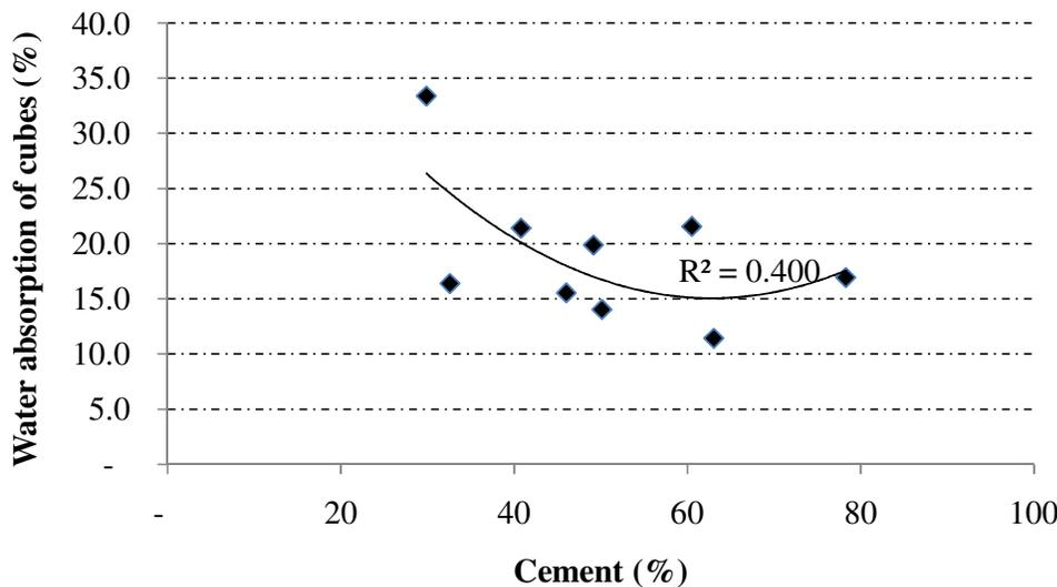
**Figure 6: Effect of cement (%) on the water absorption of cubes**
