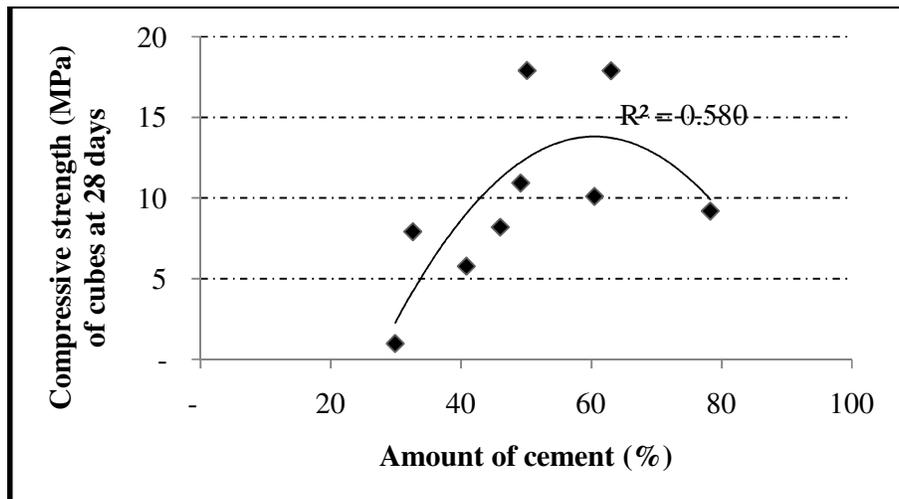
Figure 1: Effect of cement (%) on the compressive strength of cubes
