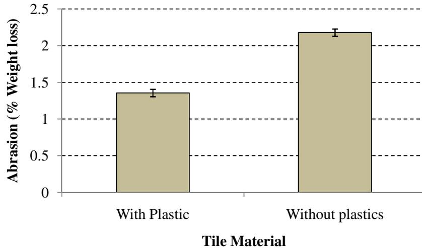
**Figure 6: Effect of plastics on abrasion**
