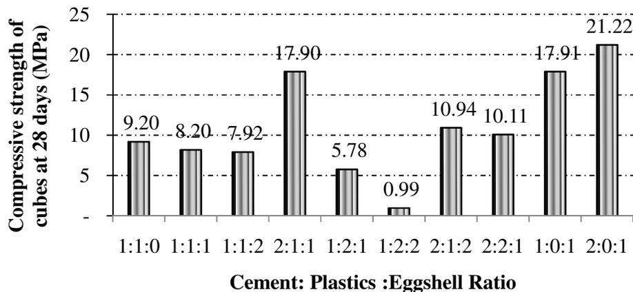
**Figure 4: Effect of the different mix ratios on compressive strength of the cubes**
