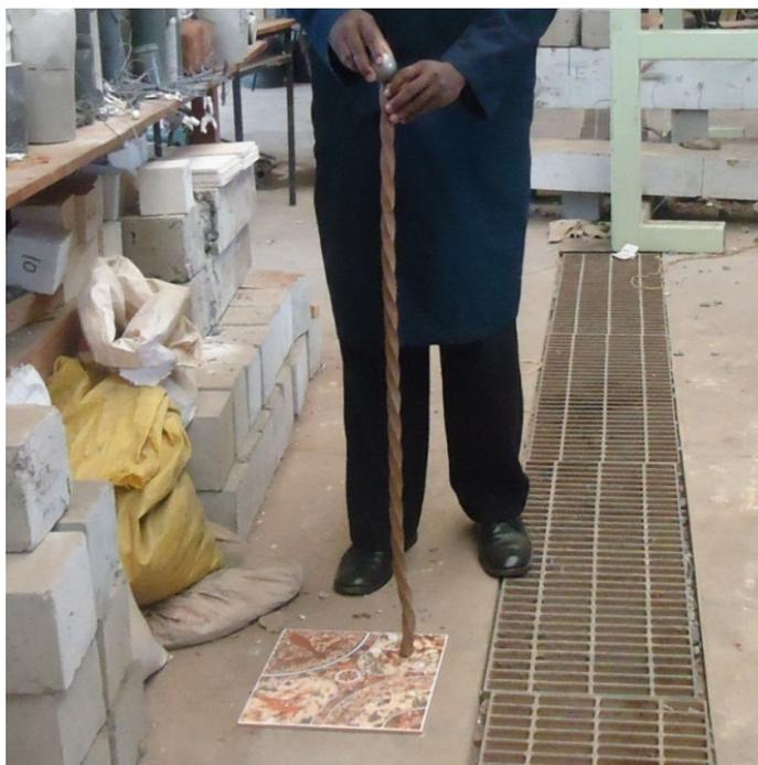
Plate 2: Spherical steel bearing dropped through one meter height
