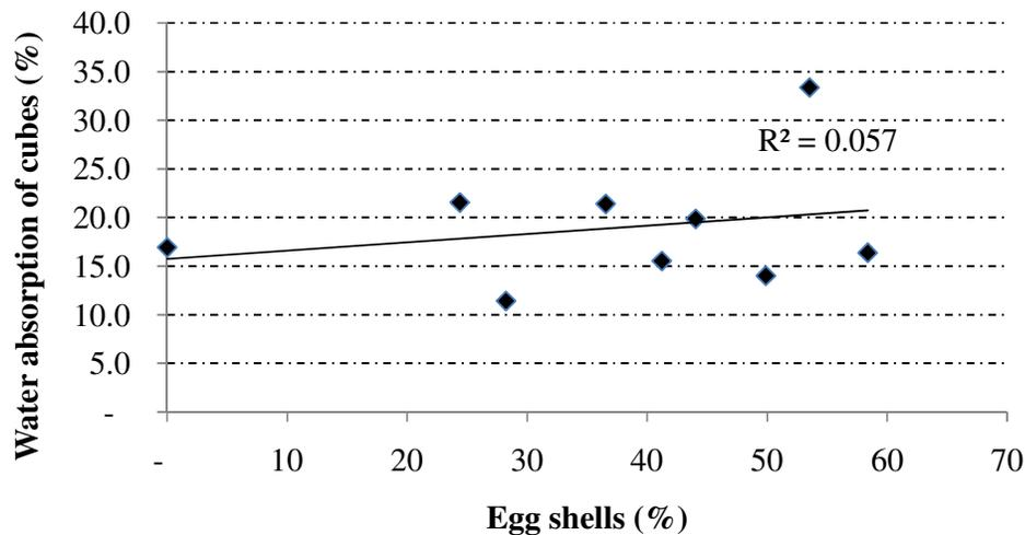
**Figure 8: Effect of egg shells (%) on the water absorption of cubes**
