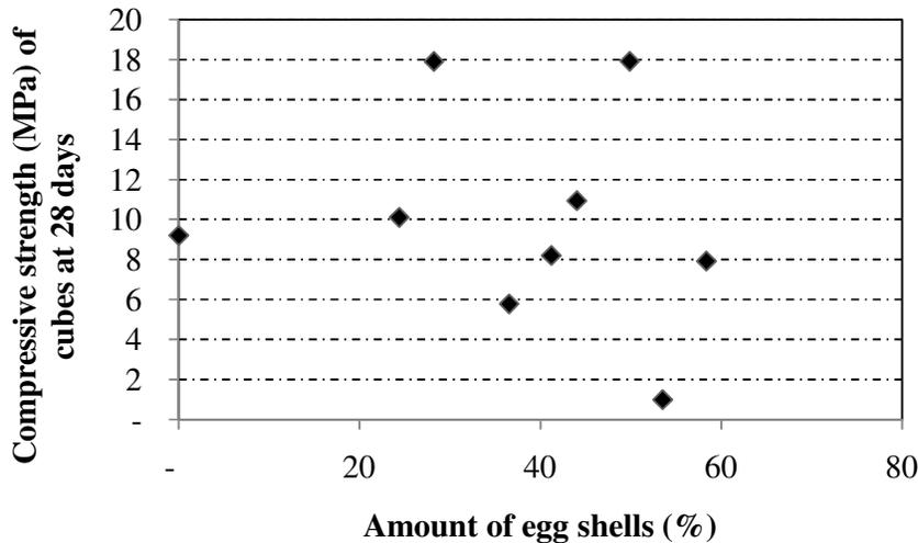
**Figure 3: Effect of egg shells (%) on the cube compressive strength**
