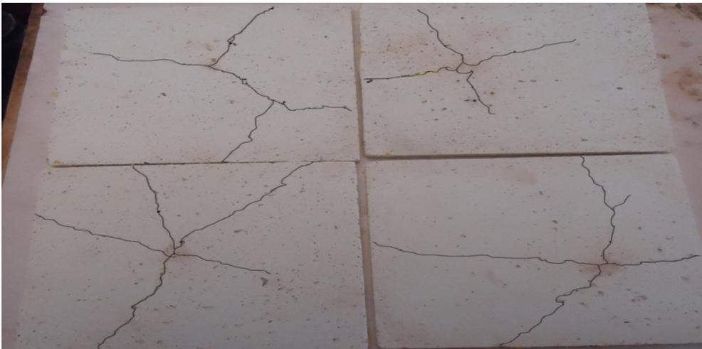
Plate 3: Indented tiles made with cement, plastics and egg shells
