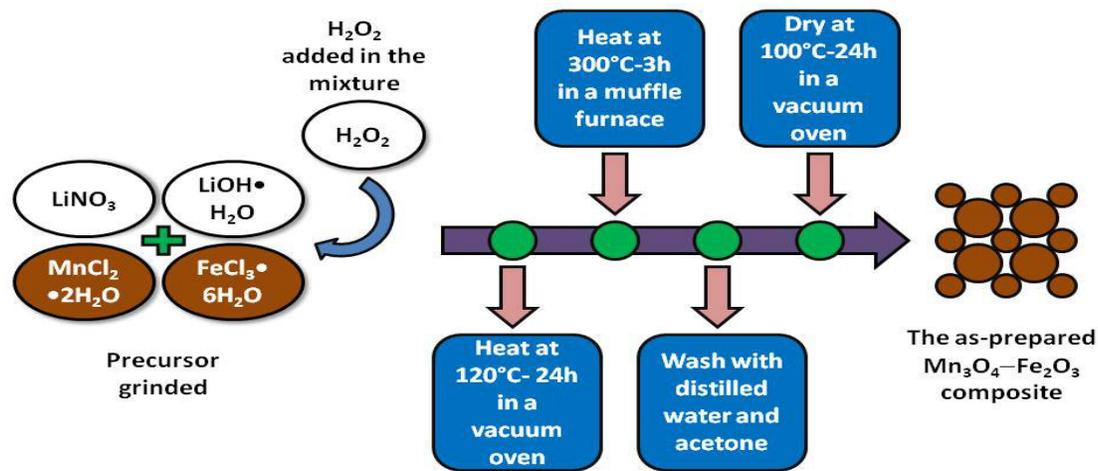
Fig. 1. Schematic diagram of a  $\text{Mn}_3\text{O}_4\text{-Fe}_2\text{O}_3$  composite formation.
