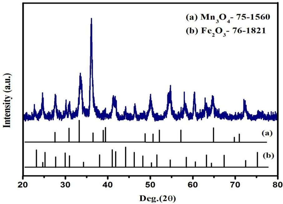
**Fig. 3.** X-ray diffraction pattern of the  $\text{Mn}_3\text{O}_4\text{-Fe}_2\text{O}_3$  composite powder synthesized under molten salt conditions.
