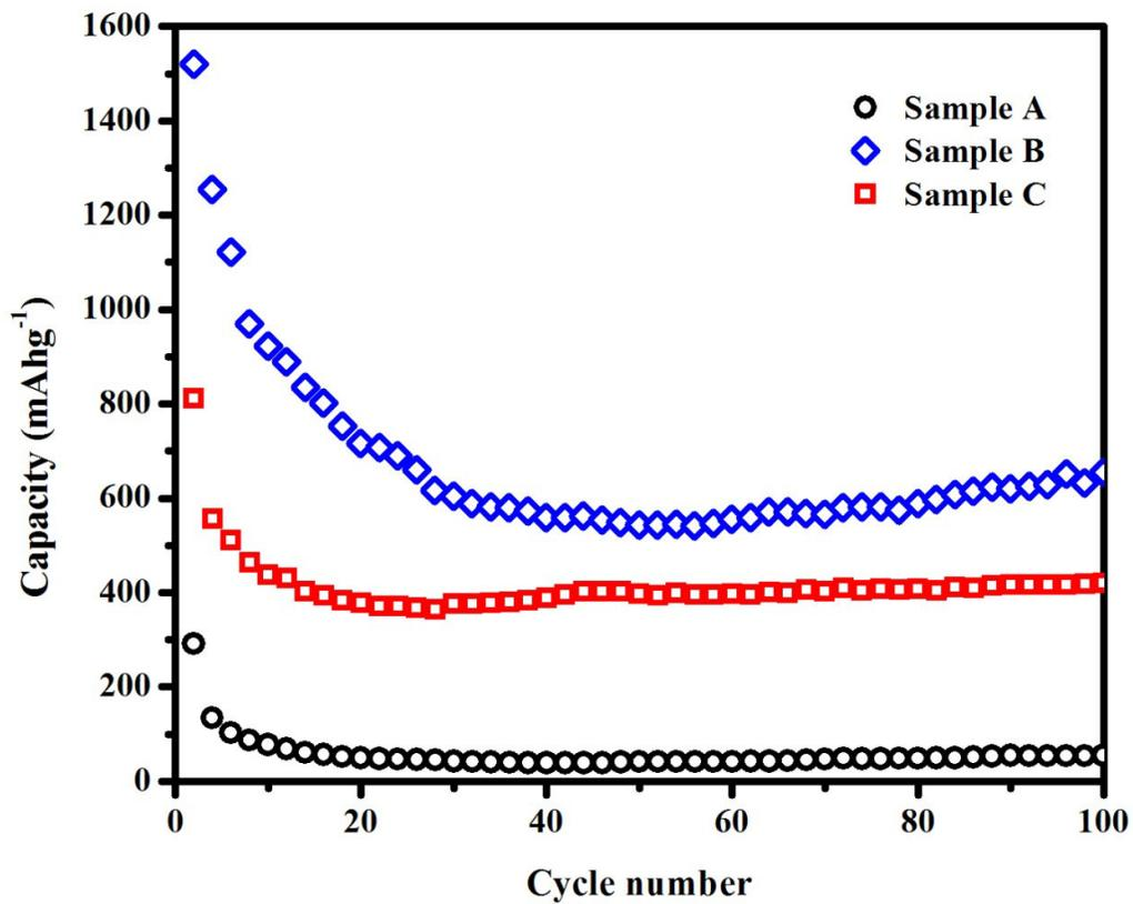
**Fig. 7.** Cycling performance of  $\text{Mn}_3\text{O}_4\text{-Fe}_2\text{O}_3$  composite anodes of sample (a) A, (b) B, and (c) C. The cells were cycled at 0.1C ( $94 \text{ mA g}^{-1}$ ).
