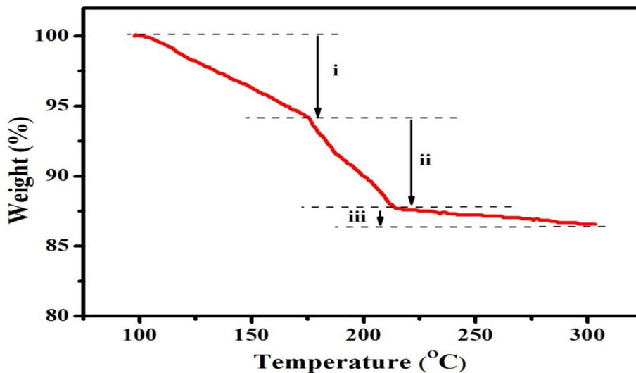
Fig. 2. TGA curve of  $\text{Mn}_3\text{O}_4\text{-Fe}_2\text{O}_3$  composite.
