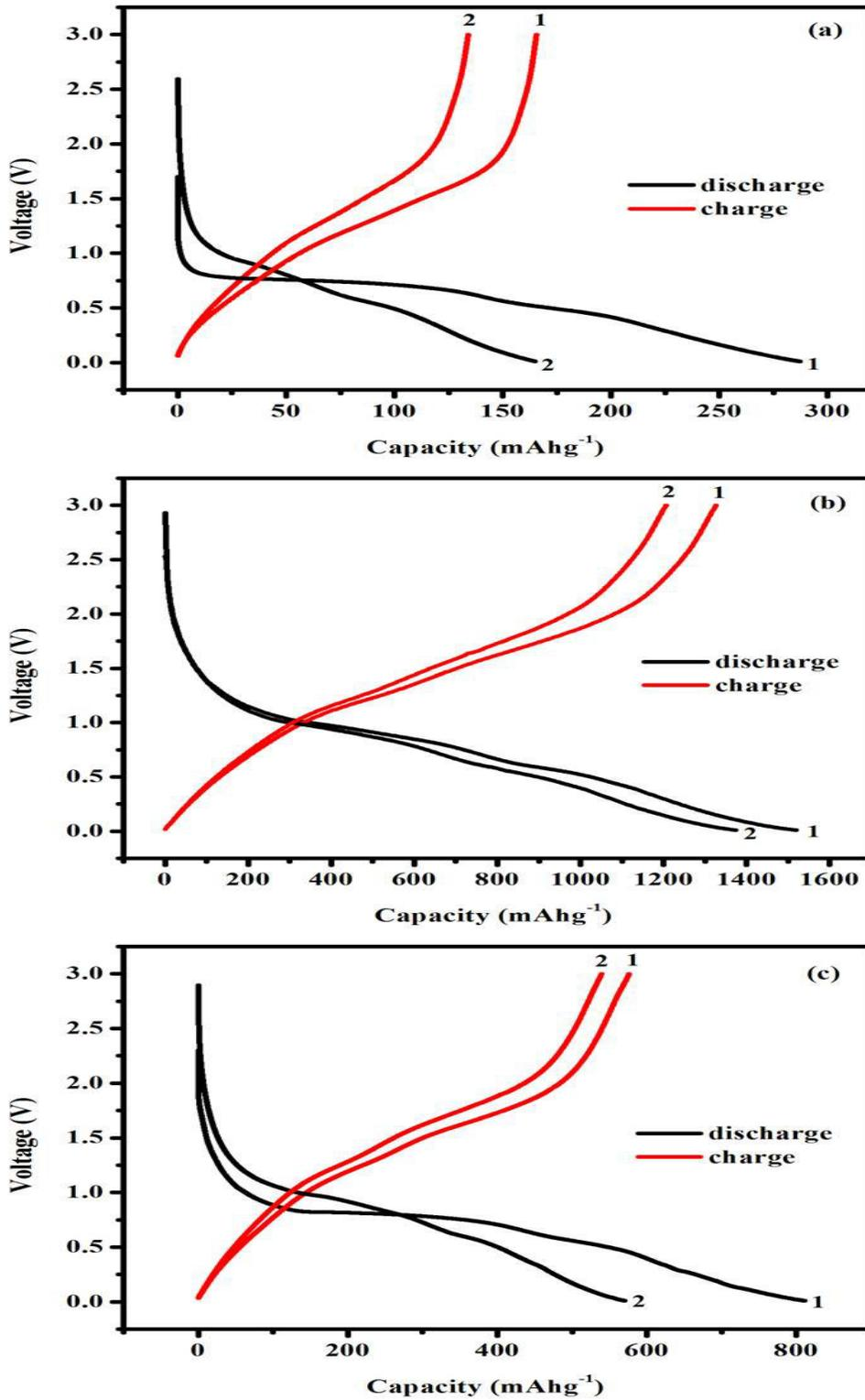
**Fig. 6.** The first and second charge-discharge profiles of Mn<sub>3</sub>O<sub>4</sub>-Fe<sub>2</sub>O<sub>3</sub> composite anode of sample (a) A, (b) B, and (c) C. The cells were charged/discharged at 0.1C (94 mA g<sup>-1</sup>).
