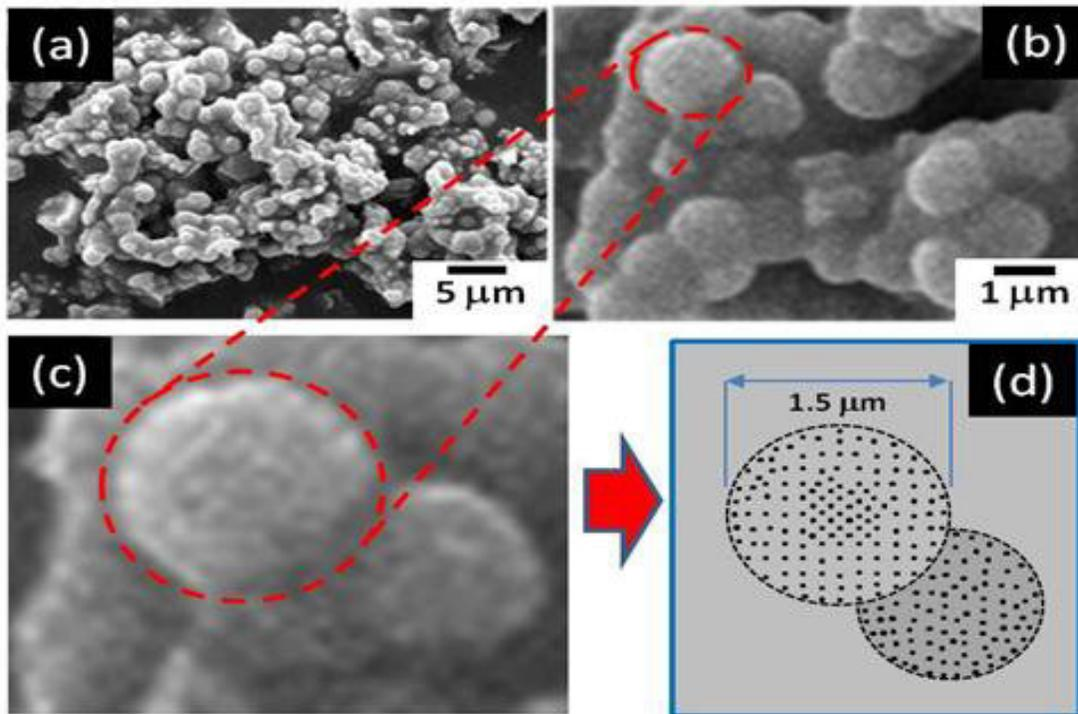
**Fig. 4.** Scanning electron microscope (SEM) images of  $\text{Mn}_3\text{O}_4\text{-Fe}_2\text{O}_3$  composite. (a) low magnification image of clusters, (b) high magnification images of clusters, (c) high magnification images of individual cluster, (d) schematic diagram of individual cluster.
