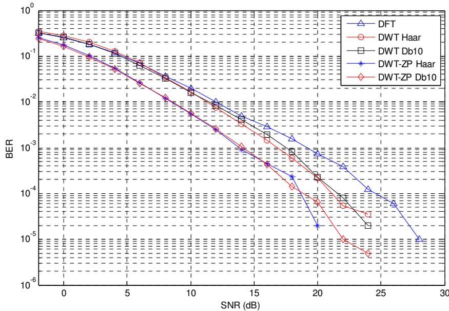
Figure 9 BER performance of 4-user MC-MC-CDMA system using DFT, DWT and DWT-ZP
