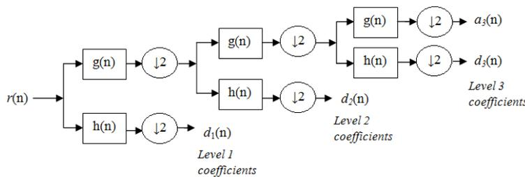
**Figure 2 Three level decomposition wavelet Transform (DWT)**
