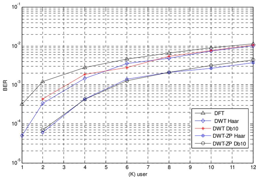
Figure 10 BER performance versus number of users (K) of MC-MC-CDMA system using DWT and DFT
