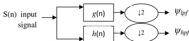
**Figure 1 Block Diagram of Wavelet Decomposition**
