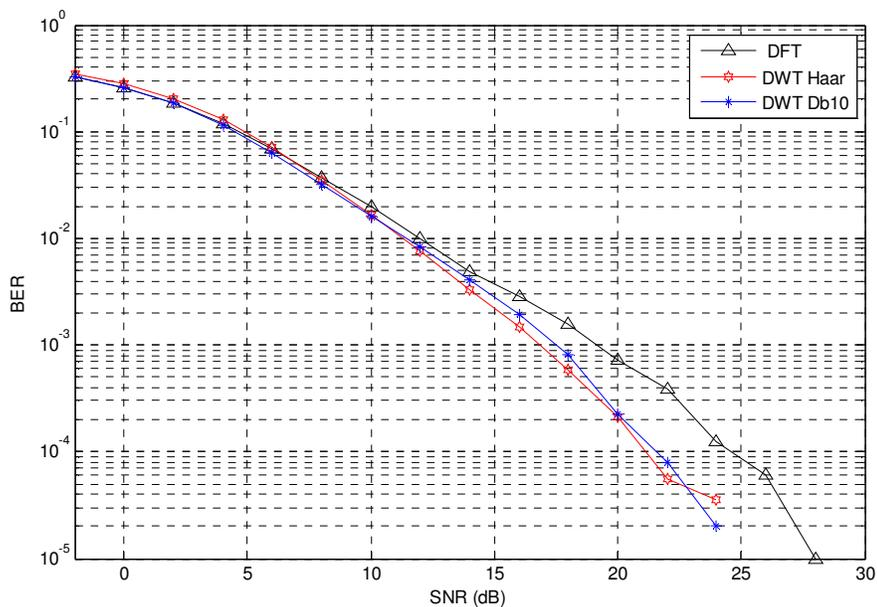
Figure 6 BER performance of 4-user MC-MC-CDMA system using DWT and DFT
