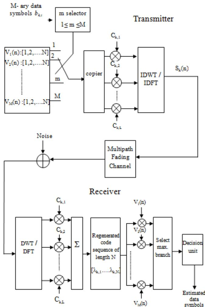
**Figure 4 MC-MC-CDMA system block diagram**
