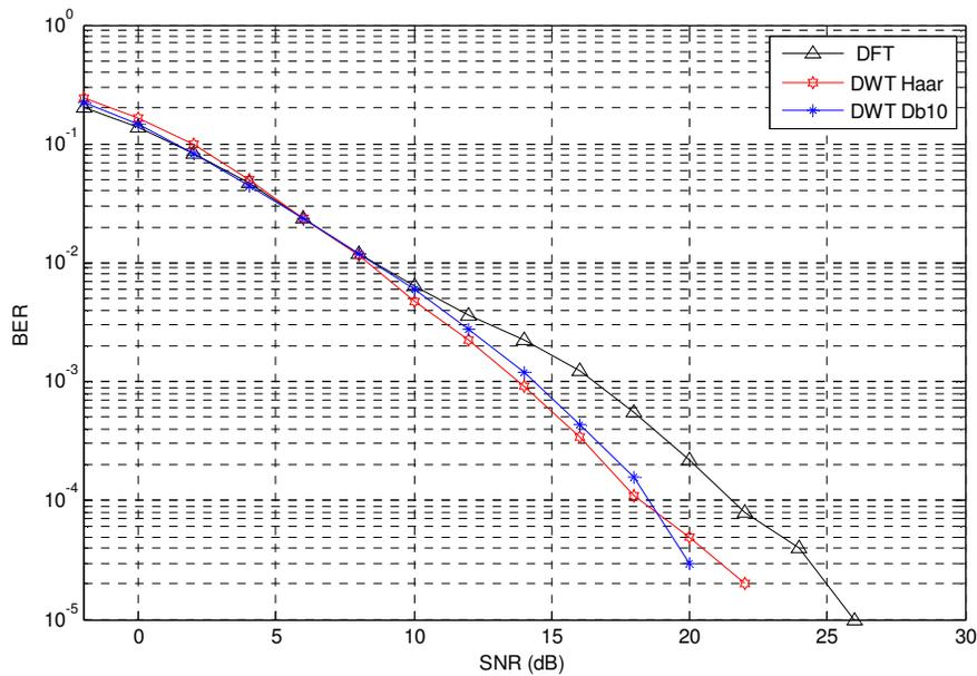
Figure 5 BER performance of 2-user MC-MC-CDMA system using DWT and DFT
