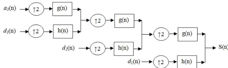
**Figure 3 Three level reconstruction wavelet Transform (IDWT)**
