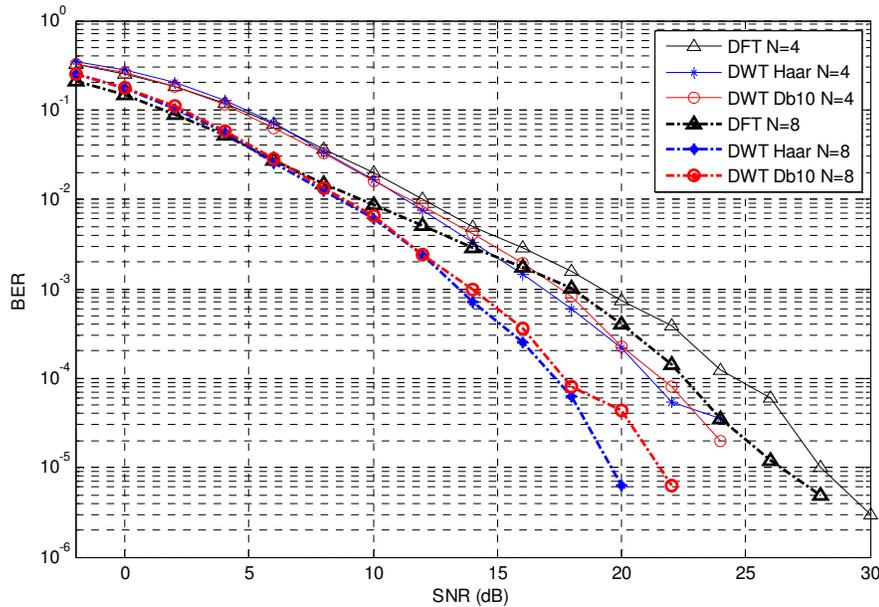
**Figure 7 BER performance of 4-user MC-MC-CDMA system using DWT and DFT with  $L=16$  and different values of  $N$**
