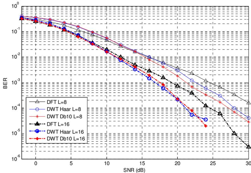
**Figure 8 BER performance of 4-user MC-MC-CDMA system using DWT and DFT with  $N=4$  and different values of  $L$**
