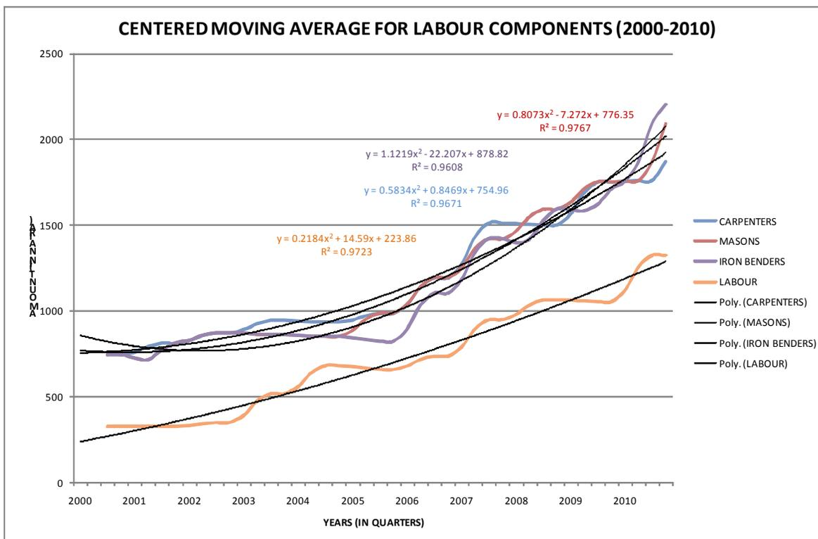
Figure 2: Model Graphs for selected Labour components
