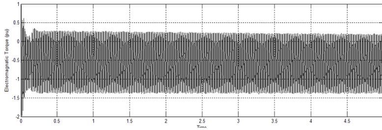
**Figure 6. Electromagnetic torque of WECS using PSF MPPT**
