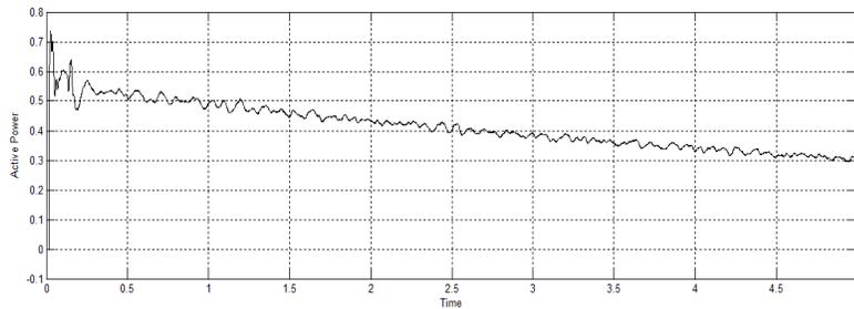
**Figure 13. Active power of WECS using HCS MPPT**
