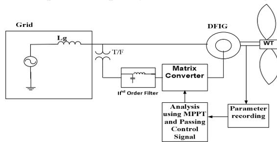
**Figure 3. Proposed Control System of WECS**
