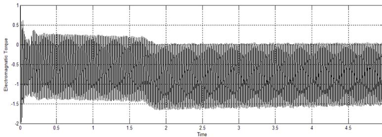
**Figure 12. Electromagnetic torque of WECS using TSR MPPT**
