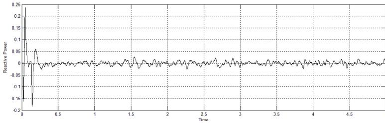
**Figure 11. Reactive power of WECS using TSR MPPT**
