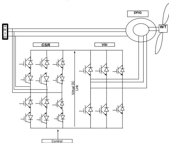
**Fig 1- Proposed WECS with Matrix Converter representation**
