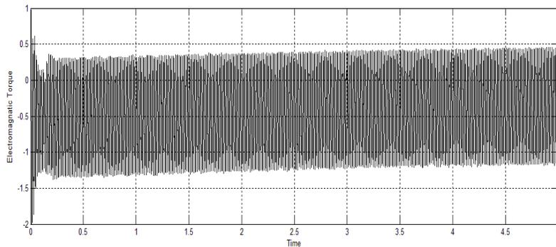
**Figure 15. Electromagnetic torque of WECS using HCS MPPT**
