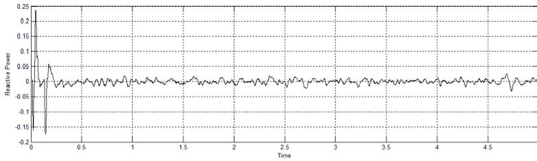
**Figure 5. Reactive power of WECS using PSF MPPT.**
