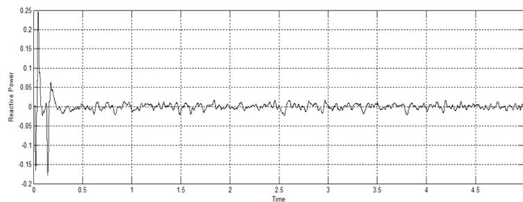
**Figure14. Reactive power of WECS using HCS MPPT**
