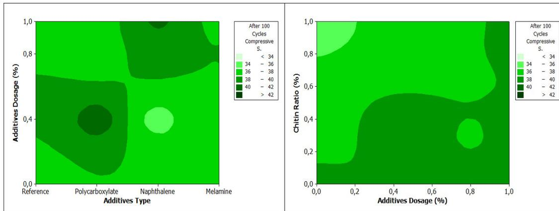
**Figure 7. The impact of (a) Additive dosage- additive type and (b) chitin ration- additive dosage on compressive strength after 100 freeze-thaw cycles**
