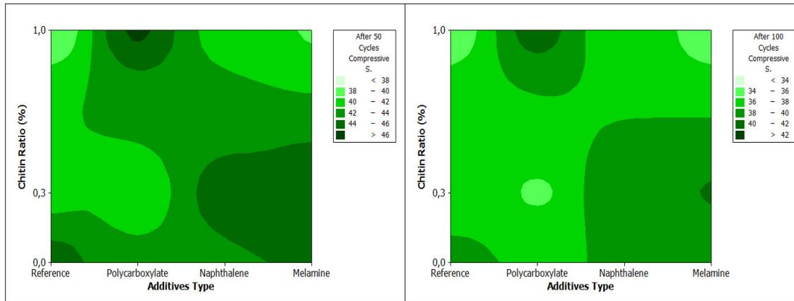
**Figure 5. The impact of additive type-chitin ratio on (a) 50 freeze-thaw and (b) 100 freeze-thaw cycles**
