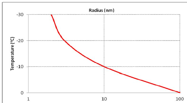
**Figure 6. The impact of capillary break diameter on freezing temperature**
