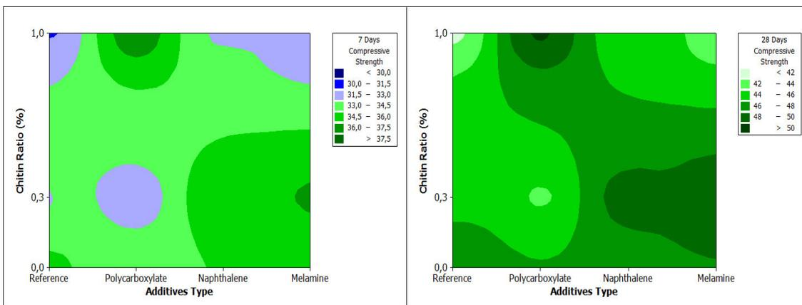
**Figure 3. The impact of chitin ratio- additive type on (a) compressive strength for 7 days and (b) compressive strength for 28 days**
