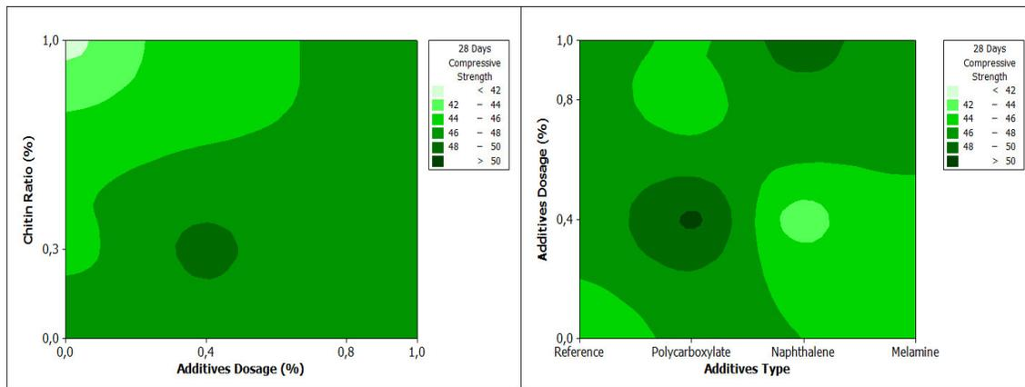
**Figure 4. The impact of (a) Additive Dosage-Chitin Ratio and (b) additive type-chitin dosage on compressive strength for 28 days**
