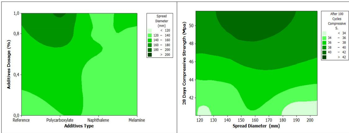
**Figure 2. (a) Additive type and the impact of dosage on flow (b) Flow diameter and the impact of compressive strength for 28 days on freeze-thaw**
