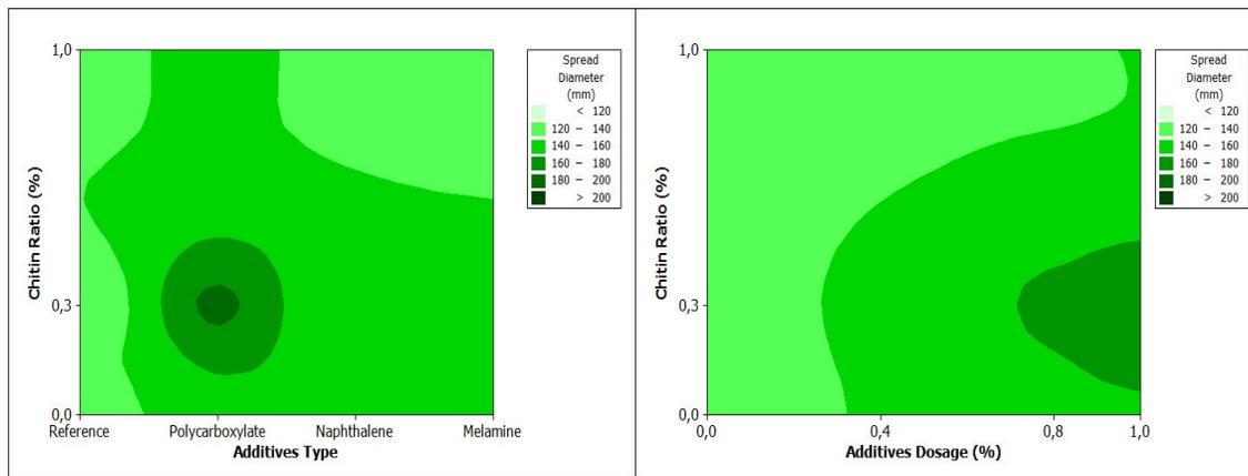
**Figure 1. (a) Chitin ratio- additive type (b) the impact of chitin ratio- additive dosage on the features of fresh mortar**
