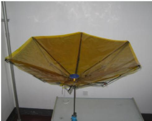
**Figure 5(a):** Deployable Antenna Actuated by Shape Memory Alloy Hinge
