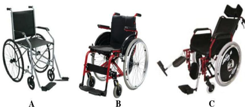
**Figure 1 - (A) Folding wheelchair with manual propulsion, (B) standard type chair, (C) semi-reclining chair.**
