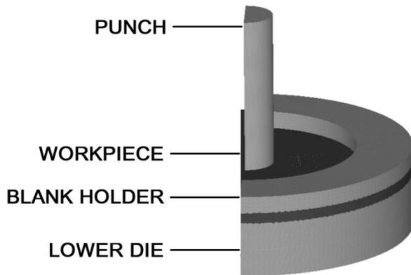
**Figure 1. The blanking set up for simulations**
