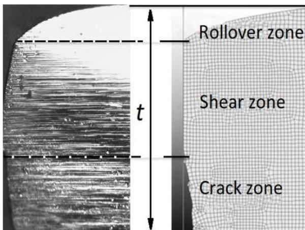
**Figure 6. Comparison of FEM and cut blank images ( $t=2$  mm)**
