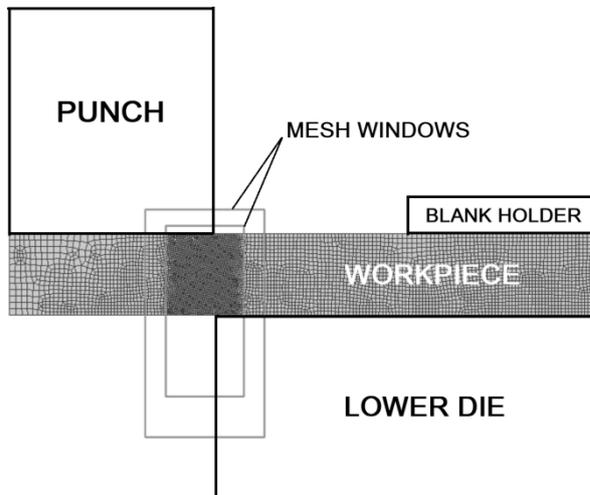
**Figure 2. Mesh distribution on the workpiece**
