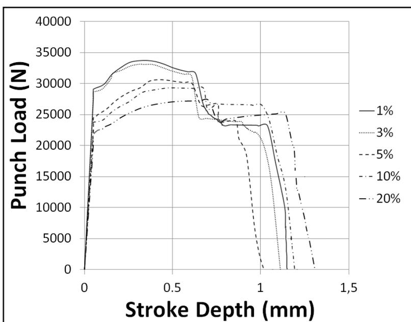
Figure 9. Punch load-stroke depth difference between two clearances
