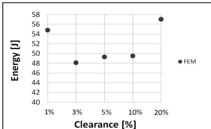
Figure 10. Cutting energy difference between clearances
