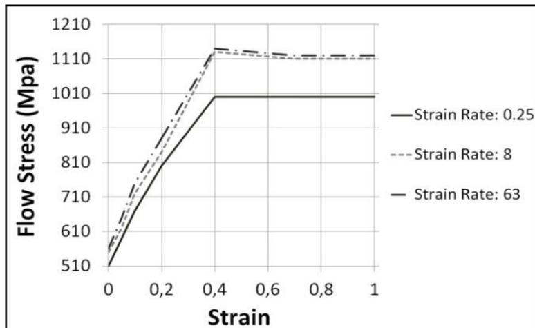
**Figure 4. The flow curve of AISI 304 according to strain rate**
