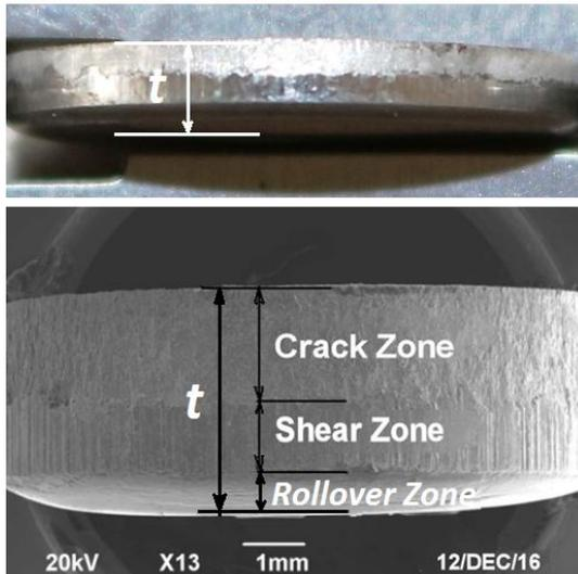
**Figure 5. Zones shown on a blank ( $t=2$  mm, clearance= 5%)**
