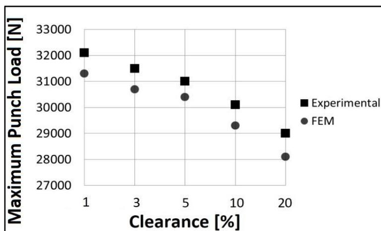
**Figure 8. Maximum punch load difference between FEM and experimental results according to clearances.**
