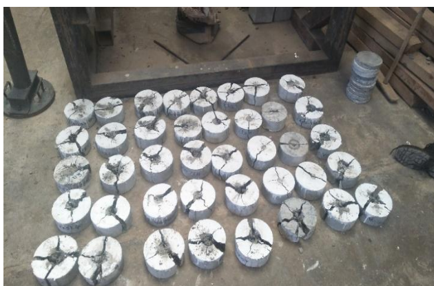
Fig. 5 Ultimate Failure mode of the spacemen
