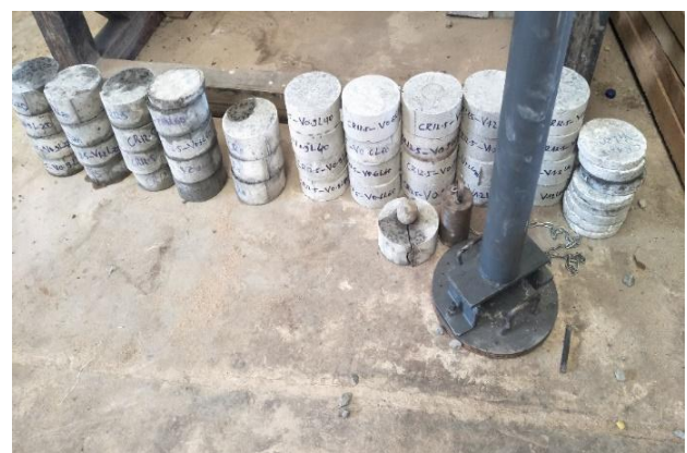
Fig.6 Sample spacemen and Impact test equipment
